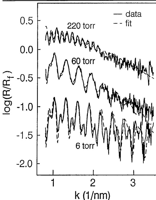
Fig. 4. Typical x-ray reflectivity spectra for samples with single Si<sub>1-x</sub>Ge<sub>x</sub> layers ( $x = 0.2\text{--}0.3$ ,  $t = 0.2\text{--}0.3$  nm) with 15 nm Si-caps. The reflected intensity is plotted as a function of scattering vector for different pressures. The solid line represents the data and the dashed line is the best fit.
