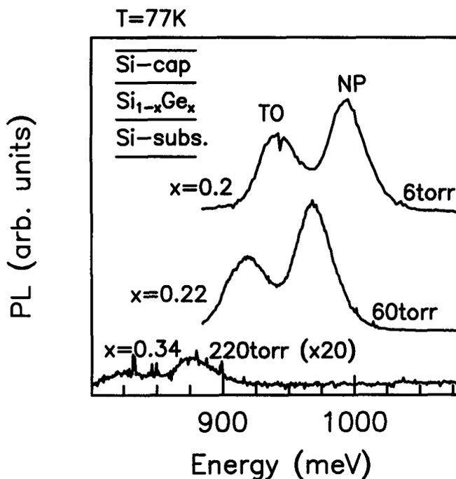
Fig. 3. Typical PL spectra of SiGe samples grown at 6, 60, and 220 Torr. Note the no-phonon (NP) peak and transverse optical (TO) phonon replica indicating band-edge luminescence and low defect concentration.
