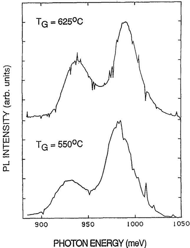
Fig. 8. Photoluminescence spectra at 77K of the single  $\text{Si}_{0.8}\text{Ge}_{0.2}$  quantum wells grown at 6 Torr, 550 and 625°C.
