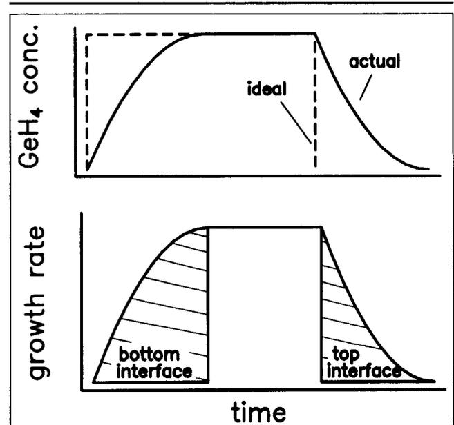
Fig. 7. A schematic diagram that explains the effects of gas switching on the thicknesses of graded layers at the top vs the bottom interface. The thickness of the interface layer is proportional to the cross-hatched area in the lower figure.
