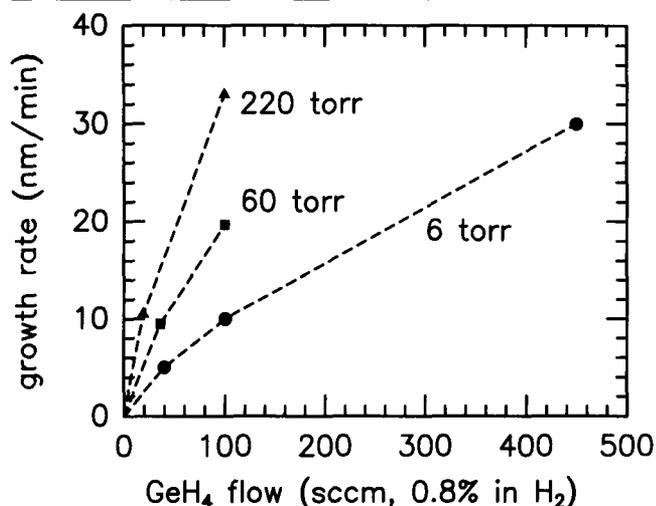
Fig. 2. Growth rate vs  $\text{GeH}_4$  flow for the same conditions as in Fig. 1. The uncertainty in growth rate is  $\pm 10\%$ .
