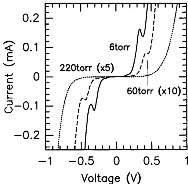
Fig. 6. Resonant tunneling diode I-V curves measured at 80K of samples grown at 6, 60, and 220 Torr. The desired structure was the same in all three samples.
