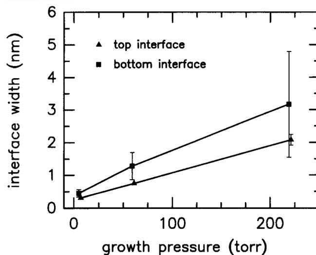
Fig. 5. The interface width of the top and bottom Si<sub>1-x</sub>Ge<sub>x</sub>/Si interfaces as a function of growth pressure.
