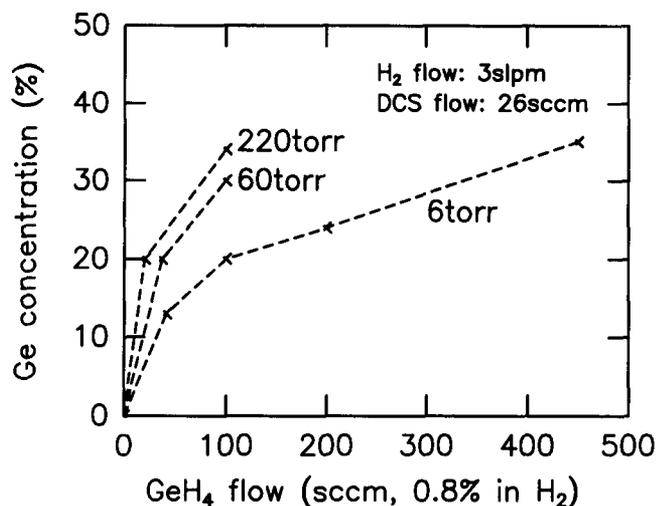
Fig. 1. Ge fraction vs  $\text{GeH}_4$  flow for different growth pressures at  $625^\circ\text{C}$ . The  $\text{H}_2$  was 3 slpm and the dichlorosilane flow was 26 sccm. The uncertainty in Ge fraction is  $\pm 2\%$ .
