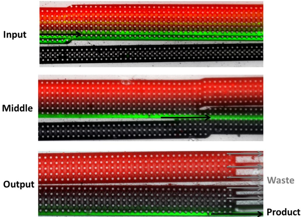
Figure 3.6: Fake color composites of fluorescent beads flowing at  $425 \mu\text{m/s}$  in DLD array with separator walls at the input, middle, and output regions.  $10\text{-}\mu\text{m}$  beads: green.  $0.2\text{-}\mu\text{m}$  beads: red.
