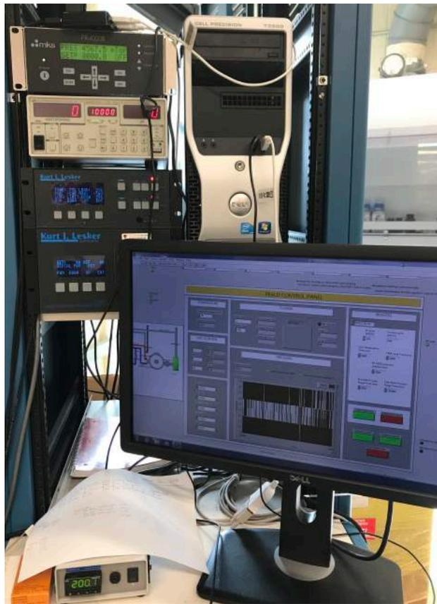
Figure 2.24: PEALD control station showing Labview interface.
