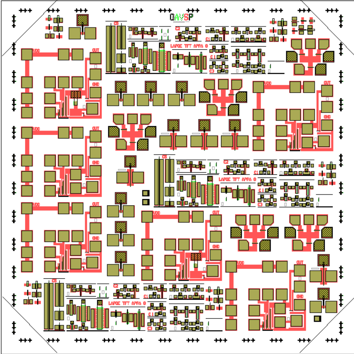
Figure B.5: Ring oscillators, test array of large TFTs and differential pairs of TFTs (with tail current source) (WRL-LargeTFTMask-Nov11.tdb)
