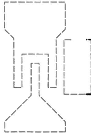
Figure B.2: Schematic layout of emitter implant, base mesa, contact hole, and metal mask used in this work. The base mesa mask was about 15 \mu\text{m} larger on each side than the outer edge of the base contact hole.
