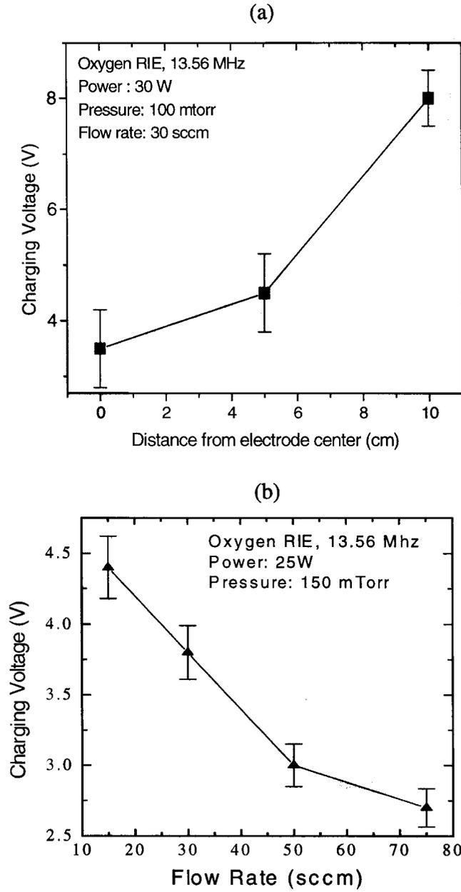
Figure 7.17 (a) Charging voltage as a function position across the electrode at constant RF power, chamber pressure and flow rate, and (b) Charging voltage as a function of flow rate of oxygen gas.
