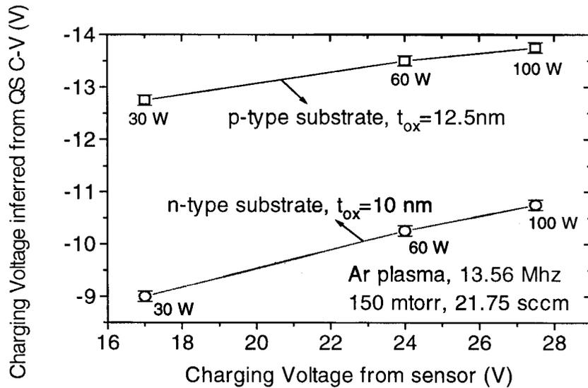
Figure 7.26. Comparison of charging voltage as measured by sensor and inferred from QS C-V degradation at different RF power.
