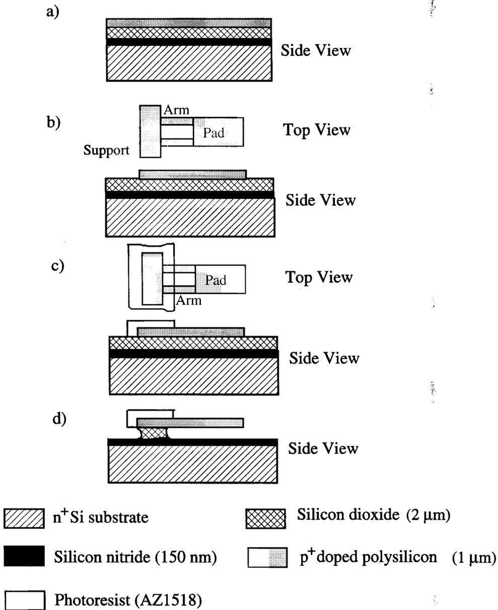
Figure 7.11. Schematic illustration of the fabrication process sequence of the paddle structure, (a) cross-section of wafer used, (b) dry etch the polysilicon, (c) spin-coat photoresist to protect the SiO<sub>2</sub> underneath the support during the release step, (d) after the SiO<sub>2</sub> underneath the paddle structure has been etched off, with the photoresist on the support to be removed by rinsing in acetone.
