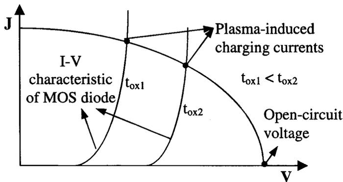
Figure 7.20. Schematic diagram of the J-V characteristics of the charging source and the charging damage seen by MOS devices with different oxide thickness exposed to it <sup>32</sup>. The MEMS charge sensor detects the open-circuit value.
