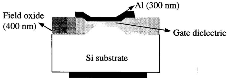
Figure 7.21. Cross-section of the capacitor used in this study, with thermal  $\text{SiO}_2$  (8-12.5 nm) as gate dielectric for MOS capacitors and, thermal  $\text{SiO}_2$  (~5 nm) and PECVD  $\text{SiN}_x$  (30-40 nm) as the gate dielectric for the MNOS capacitors.
