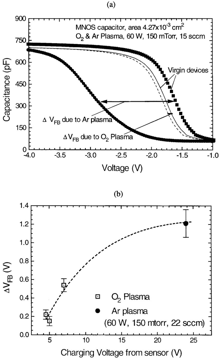
Figure 7.27. (a) High frequency C-V curves of MNOS capacitors before and after exposure to argon and oxygen plasmas. (b) Illustration of the correlation of flat-band voltage shift of MNOS capacitors, after plasma treatment with charge sensor reading.
