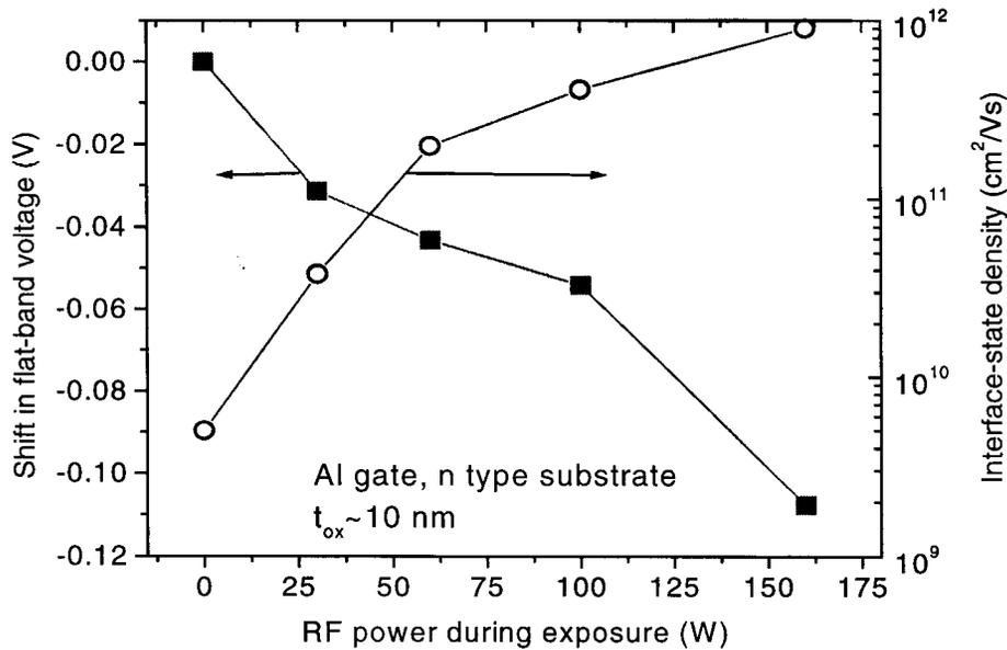
Figure 7.23. Shift in flat-band voltage and change in interface-state density of MOS capacitors after argon plasma exposure at different RF powers.
