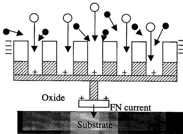
Figure 7.3. Schematic cross-section at a moment near endpoint of dense-line pattern etching, showing the electron shading effect, with anisotropic ions reaching the spaces while the isotropic electrons are shielded by the mask. The open circles represent ions, and the closed symbols electrons <sup>5</sup>.
