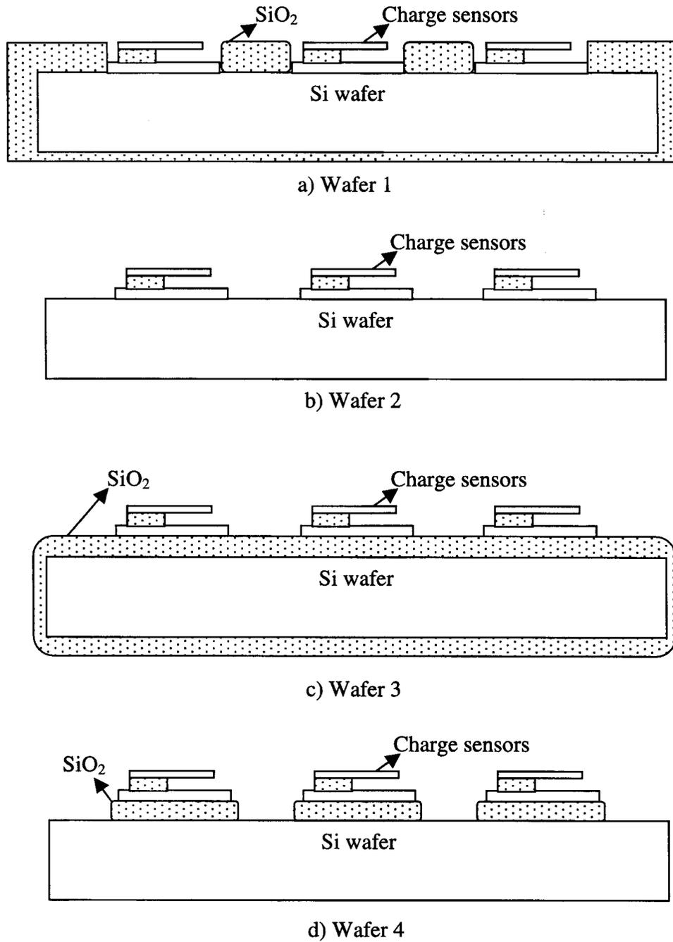
Figure 7.19. Schematic cross-sectional illustrations of the different configurations used to bond the sensors on to the Si wafer to study the charging across a 100-mm Si wafer, when exposed to  $\text{O}_2$  plasma at 60 W, pressure of 150 mtorr and an oxygen flow of 15 sccm.
