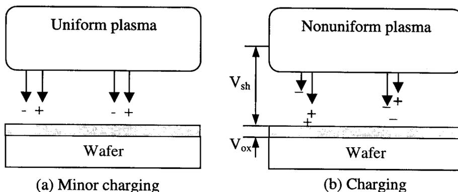
Figure 7.1. A schematic model showing the wafer charging for oxide exposed to (a) an uniform plasma, and (b) oxide exposed to a nonuniform plasma at the initial state, where  $V_{sh}$  is the sheath voltage, and  $V_{ox}$  is the oxide voltage <sup>6</sup>.
