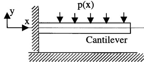
where  $y$  is the deflection (height) cantilever,  $E$  is the Young's modulus of elasticity of the beam,  $p$  is the electrostatic force at each point due to the applied bias, and  $I$  is the moment of inertia about the neutral axis of deflection. The boundary condition is that the deflection at the fixed end is zero.  $I$  for a cantilever is given by  $bt^3/12$  where  $b$  is the
