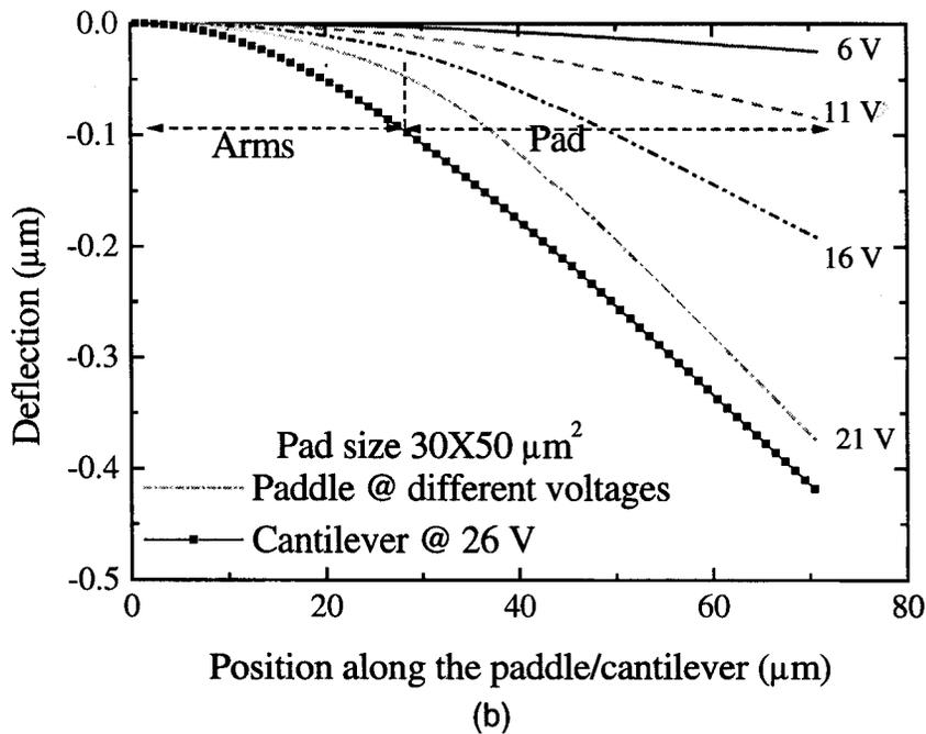
Figure 7.9. Simulation results of the paddle structure, (a) tip deflection angle as a function of the voltage bias between the polysilicon and the substrate for various sizes of paddles, and (b) side-view of the deflection of the paddle structure at various biases with the deflection of the cantilever shown for comparison.
