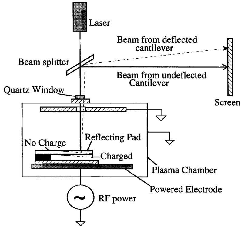
Figure 7.14. Schematic illustration of the set-up used to detect plasma induced charging on the surface directly and non-invasively through measurement of the shift in the laser reflected spot.
