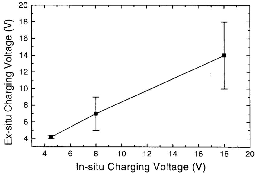
Figure 7.15. Comparison of charging voltage measured by the in-situ direct method (from laser deflection) and that measured by the ex-situ method (from inspecting the paddles after exposure).
