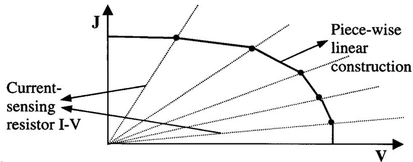
Figure 7.5. CHARM-2 charge sensors with different value of charge-sensing resistors allowing the reconstruction of the  $J$ - $V$  characteristics of the charging source <sup>15</sup>.
