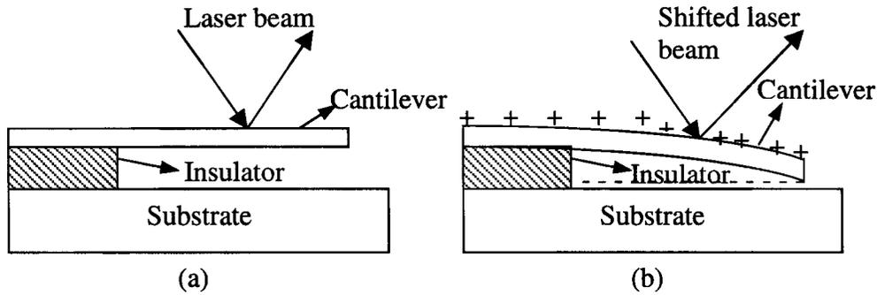
Figure 7.6. Microscopic charge-sensing structure for (a) uncharged and (b) charged surfaces.
