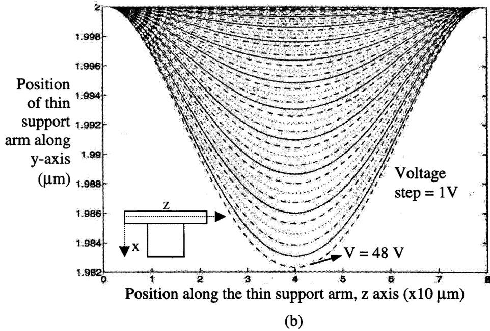
Figure 7.10. Simulation results of the torsional mirror structure, (a) tip deflection angle as a function of the voltage bias between the polysilicon and the substrate, and (b) side-view of the deflection of the support arm for various biases.
