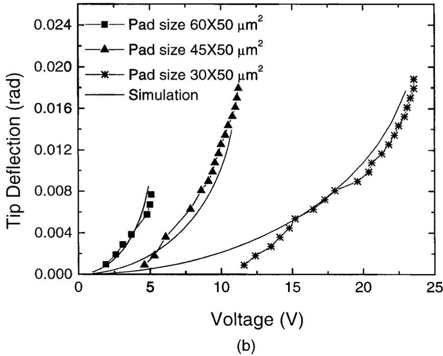
Figure 7.13. (a) Schematic diagram of the set-up used to calibrate the charge sensors externally, and (b) the tip deflection angle as a function of the applied bias between the polysilicon and the substrate for various sizes of paddles, with both the measured and the simulated data shown.
