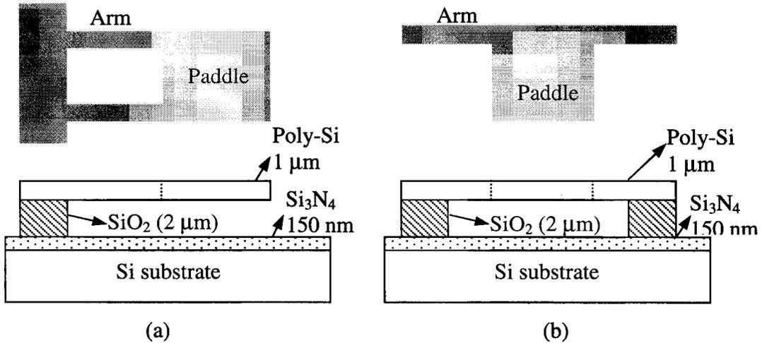
Figure 7.7. Schematic diagram of the top and side views of (a) paddle structure, and (b) torsional mirror, with the thickness of the different layers indicated.
