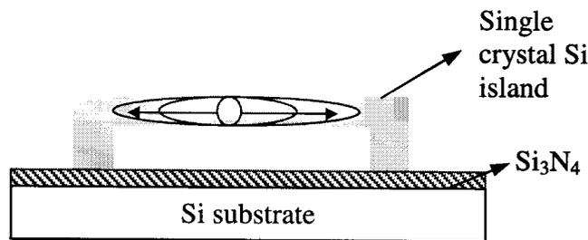
b) Remove all  $SiO_2$  and anneal at  $\sim 600^\circ C$  to realize defect-free single crystal Si island.
