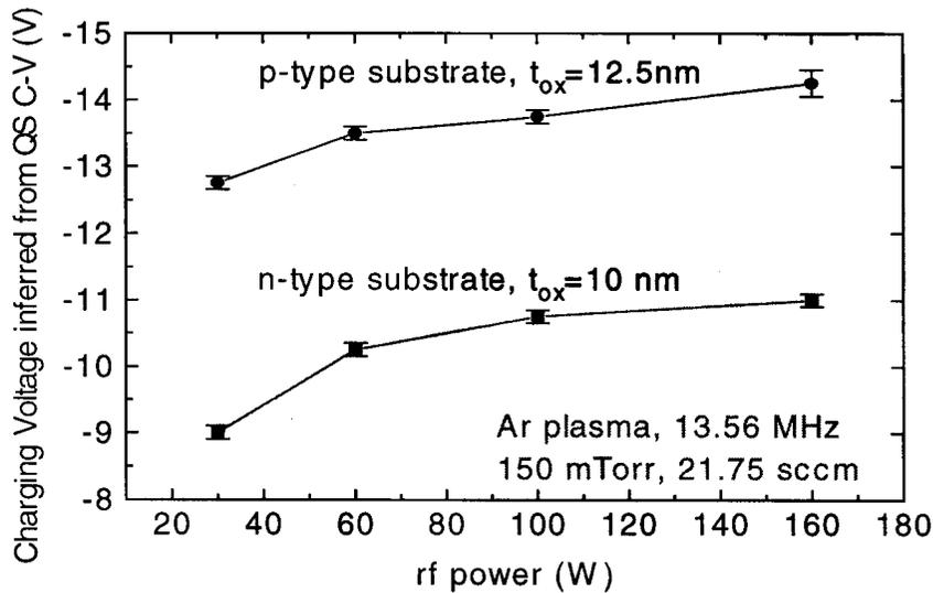
Figure 7.25. Charging voltage across the oxide during argon plasma exposure inferred from DC bias stressing and matching the QS C-V curves for n & p type substrate MOS capacitors.
