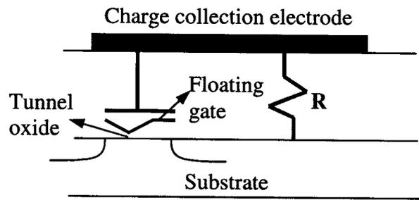
Figure 7.4. Schematic diagram of the cross-section of the CHARM-2 charge sensor with a resistor connected in parallel to the EEPROM transistor between the charge collection electrode and the substrate <sup>15</sup>.
