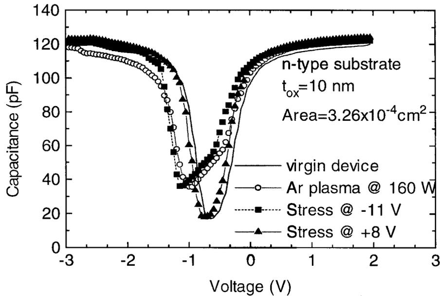
Figure 7.24. Comparison of QS C-V curves of devices exposed to argon plasma at RF power of 160 W and DC bias stressed externally for the same duration.
