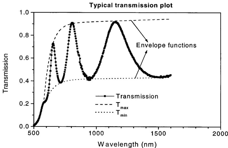
Figure B.2. Transmission of light through a thin film as function of wavelength of light. The maxima and minima occur because of constructive and destructive interference.
