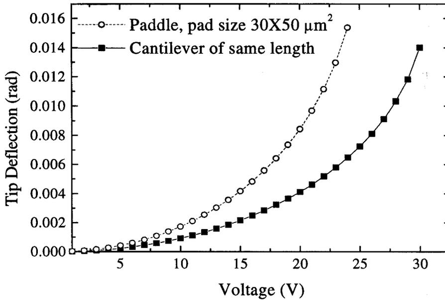
Figure 7.8. Tip deflection vs. voltage for the paddle structure and a simple cantilever of the same length (simulated).
