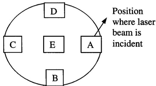
Figure 7.18. Schematic diagram of a 100-mm Si wafer showing the positions of the charge sensors.
