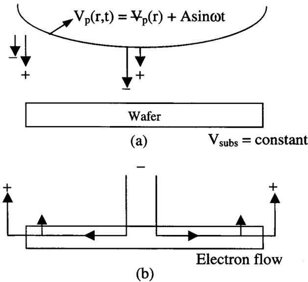
Figure 7.2. A schematic diagram showing (a) how the local ion/electron current imbalance occurs from a nonuniform plasma.  $J_e$  is larger at the wafer center than at the edge because of the smaller electron barrier ( $V_{sh}$ ) at the center, and showing (b) electron flow across the entire wafer at steady state <sup>16</sup>.
