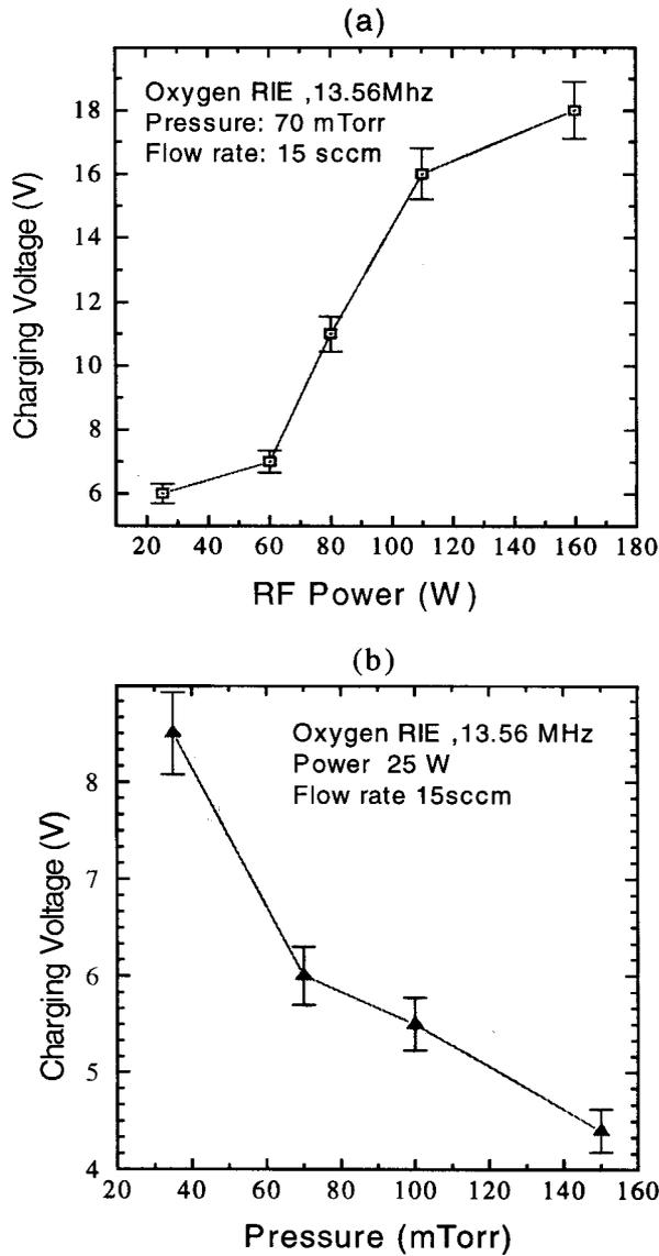
Figure 7.16. (a) Charging voltage as a function of input RF power at constant flow rate and chamber pressure, and (b) charging voltage as a function of chamber pressure at constant flow rate and RF power.
