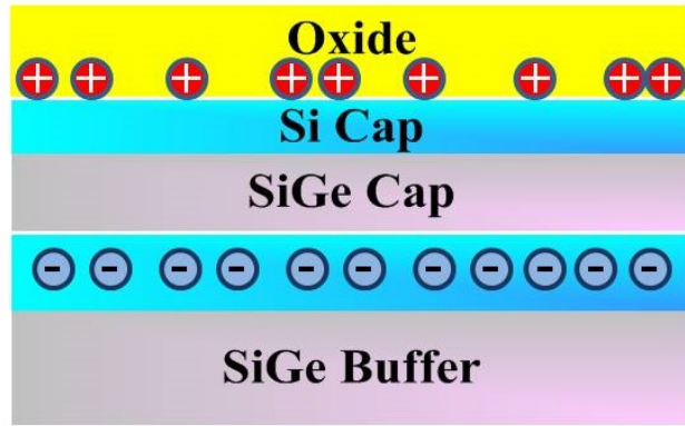
Figure 5.2: The schematic of remote charged impurities at the oxide/silicon interface in an undoped silicon 2DEG.
