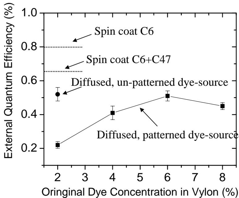
**Figure 2-24.** EL quantum efficiencies of green devices fabricated with different dye doping methods. [29]
