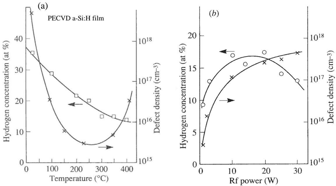
**Figure 3-6.** Defect density and hydrogen concentration in a-Si film as a function of (a) substrate temperature and (b) rf power during PECVD process [1].
