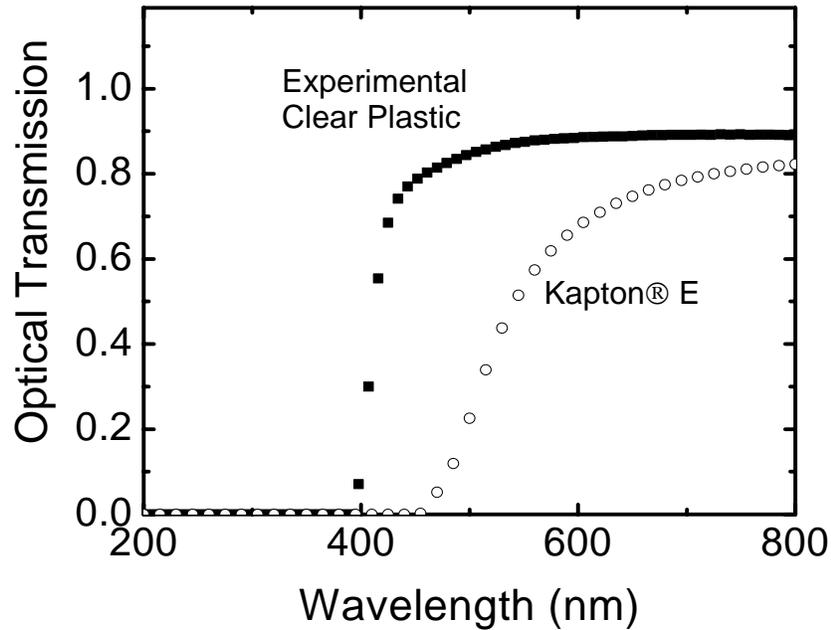
**Figure 4-1.** . Optical transmission spectra of a 50µm-thick foil of Kapton® 200E and of a 75µm-thick clear plastic substrate A .
