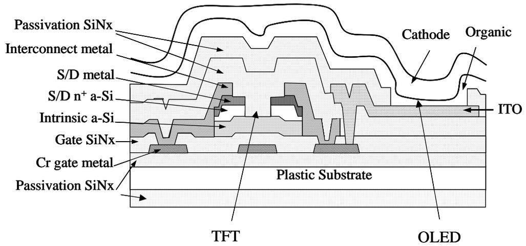
**Figure A-2.** Schematic cross-section of the TFT-OLED integration on clear plastic substrate.
