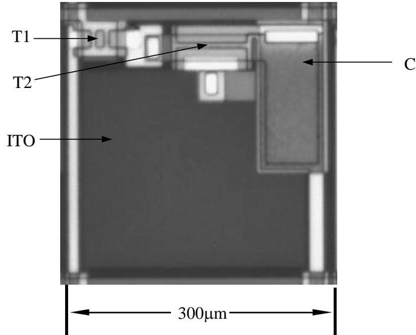
**Figure 5-5.** Micrograph of a pixel in a 2-TFT AMOLED array before OLED integration. T1 is the switching transistor, T2 the drive transistor, and C is the storage capacitor. The patterned ITO will become the anode of the OLED.
