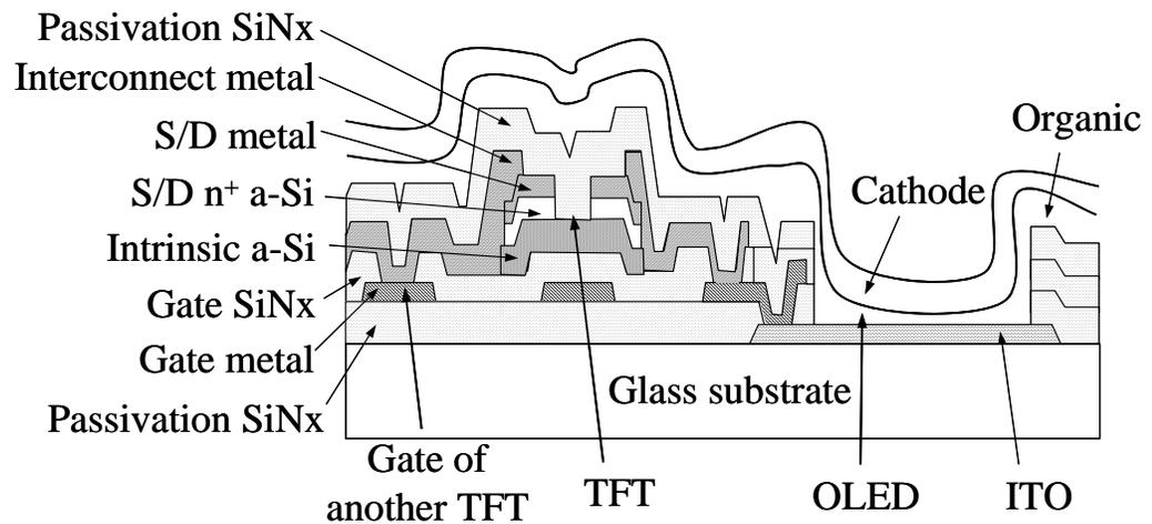
**Figure A-1.** Schematic cross-section of the TFT-OLED integration on ITO/glass substrate.
