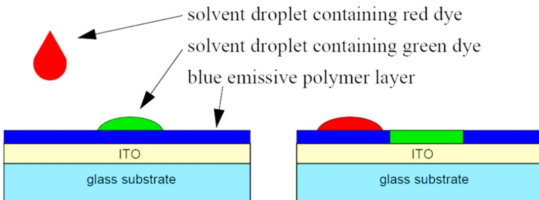
**Figure 2-5.** Patterning of the emission color by local ink-jet printing of dye solution.
