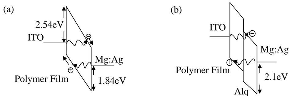
**Figure 2-15.** Reverse-biased band diagrams of the (a) single-layer (90nm PVK/PBD/Dye) and (b) bi-layer (90nm PVK/PBD/Dye + 40nm  $\text{Alq}_3$ ) OLED's. The diagram shows tunneling. Reduction in current would also be expected for emission over a barrier. [26]
