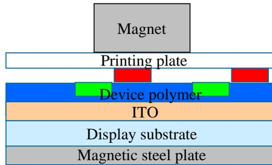
**Figure 2-9.** Schematic cross section of the aligned magnetic steel plate, device plate, dye source plate and magnet stack ready for putting in the oven for dye transfer. Vertical dimensions are exaggerated over lateral dimensions.
