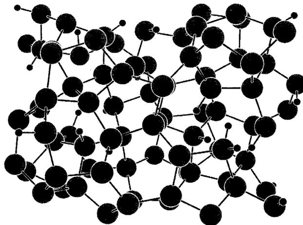
**Figure 3-1.** Model of the atomic structure of a-Si:H showing the random covalent network and the Si-H bonds. [6]
