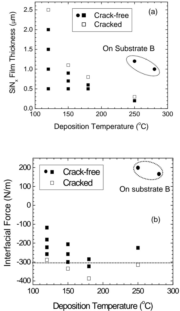
**Figure 4-5.** (a) Thickness and (b) Interfacial force of cracked (open symbols) and crack-free (filled symbols) SiN<sub>x</sub> films deposited over a range of temperatures. The two films on substrate B (with low CTE) are labeled separately.
