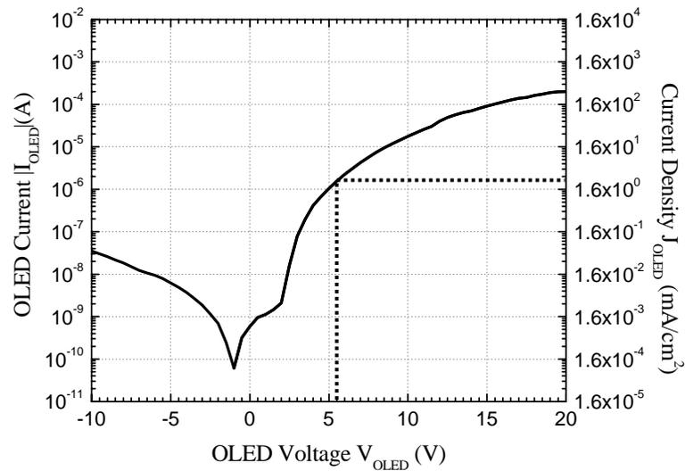
**Figure 5-12.** I-V characteristics of a test OLED with an area of  $250\mu\text{m} \times 250\mu\text{m}$ . Dotted lines show current density needed for  $200 \text{ cd/m}^2$  OLED brightness.
