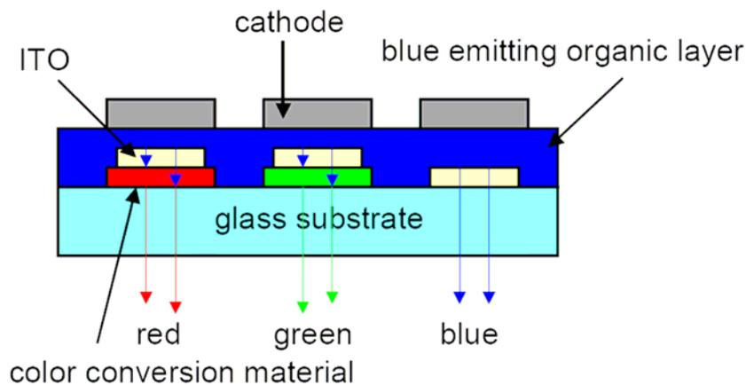
**Figure 2-4.** RGB emission using blue OLED and color conversion materials.
