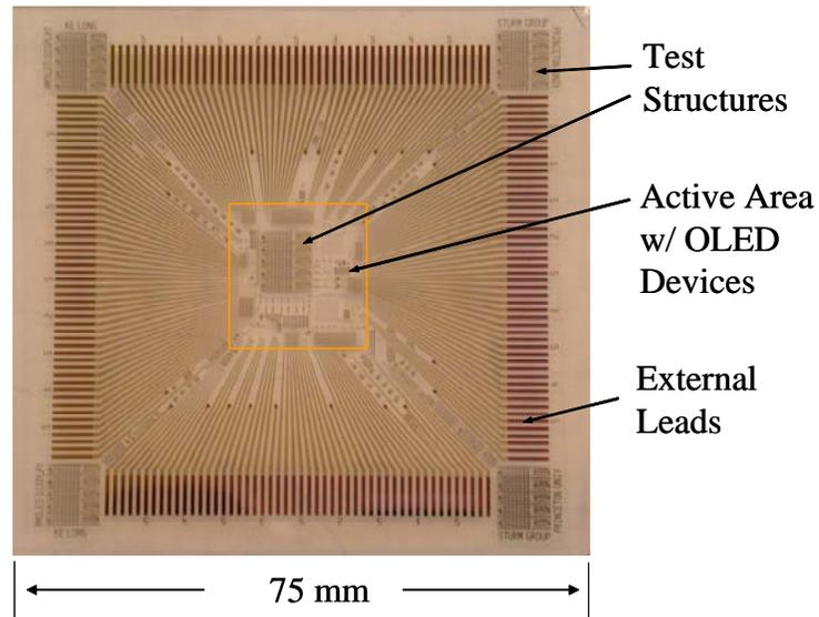
**Figure 5-3.** Photograph of a test sample. The TFT driving circuits are fabricated, waiting for OLED integration.
