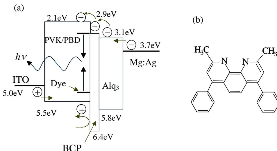
**Figure 2-19.** (a) Schematic band diagram of the tri-layer OLED structure with PVK:PBD:Dye/BCP/Alq<sub>3</sub>. The electric fields are omitted (i.e. the bands are drawn flat) to show more clearly the relative energy levels in the different materials and how the HOMO in the BCP blocks holes from reaching the Alq<sub>3</sub>. (b) Chemical structure of 2,9-dimethyl-4,7-diphenyl-1,10-phenanthroline (BCP). [29]
