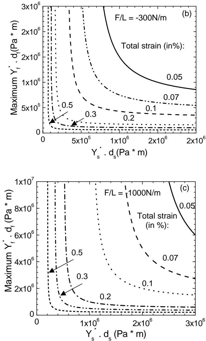
**Figure 4-7.** Calculated maximum allowed products of device layer thickness times its Young's modulus ( $d_f \cdot Y_f^*$ ) vs. the substrate thickness times its Young's modulus ( $d_s \cdot Y_s^*$ ), for a range of values of the total strain level in the film. The critical interfacial force is assumed to be (a)  $-100 \text{ N/m}$  (on previous page); (b)  $-300 \text{ N/m}$ ; (c)  $-1000 \text{ N/m}$ .
