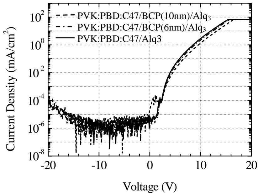
**Figure 2-21.** I-V characteristics of the blue dye-doped OLED devices with or without BCP hole/exciton blocking layer. [26]
