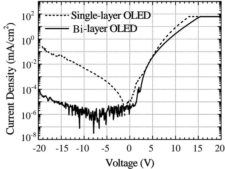
**Figure 2-16.** Typical I-V characteristics of the single-layer (dashed line) and bi-layer (solid line) devices doped with green dye C6, where the PVK/PBD/C6 layer is made by spin-coating. [29]
