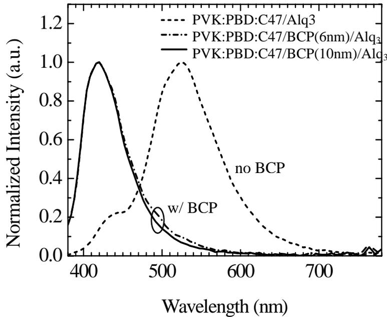
**Figure 2-20.** Electro-luminescence spectra of the blue dye-doped OLED devices with or without BCP hole/exciton blocking layer. [29]
