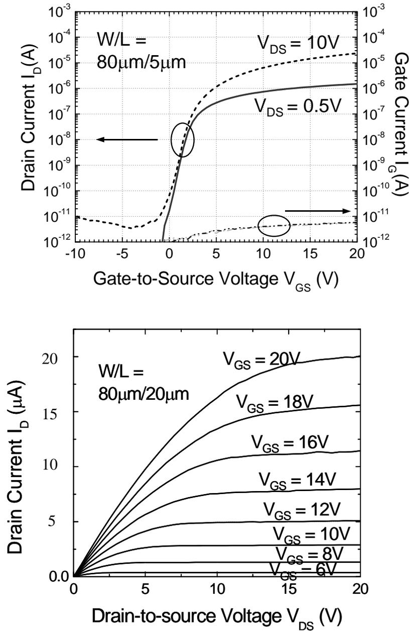
**Figure 4-12.** Transfer (a) and output (b) characterizations of a-Si TFT's made on glass with a maximum process temperature at  $180^\circ\text{C}$ .
