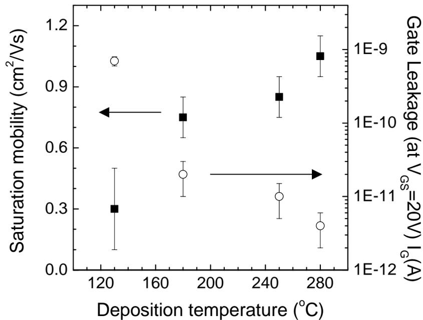
**Figure 4-14.** Saturation mobilities and gate leakage currents of TFT's made at different maximum process temperatures. Size of the TFT's are W/L = 80μm/40μm. [25]
