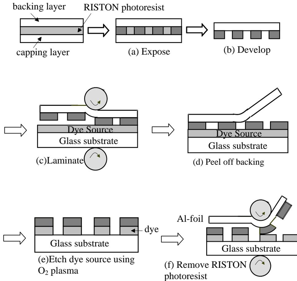
**Figure 2-8.** Fabrication of the printing plate. (a) pattern RISTON dry photoresist with backing layer remaining as support; (b) laminate patterned RISTON dry photoresist onto the surface of the dye-doped polymer layer (together with backing layer); (c) peel off the backing layer to expose the pattern on the dry photoresist; (d) etch dye-doped polymer using oxygen plasma; (e) remove the dry photoresist by laminating to and peeling off with an aluminum foil. [21]
