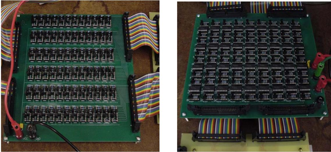
Figure A-4. Pictures of the row driver and column driver PCB.
