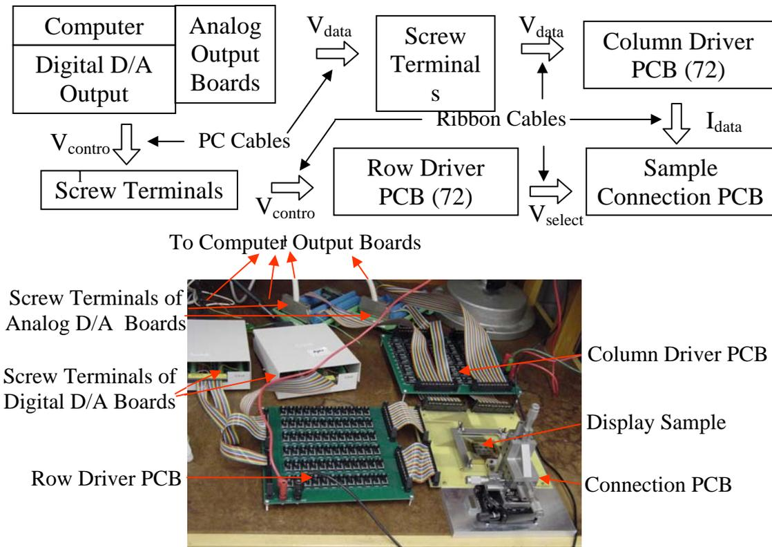
Figure A-6. Schematic of the driving setup.
