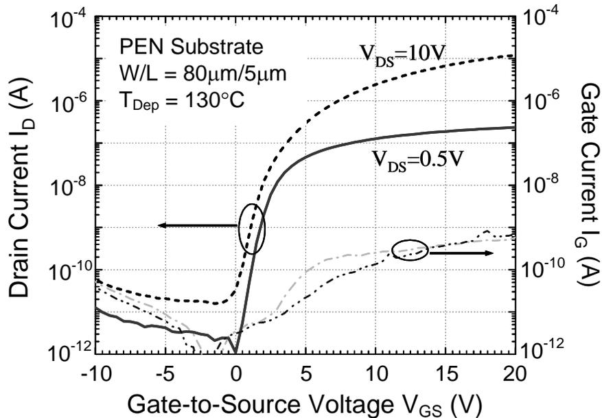
**Figure 4-2.** Transfer characteristics of a TFT processed at 130°C on PEN.
