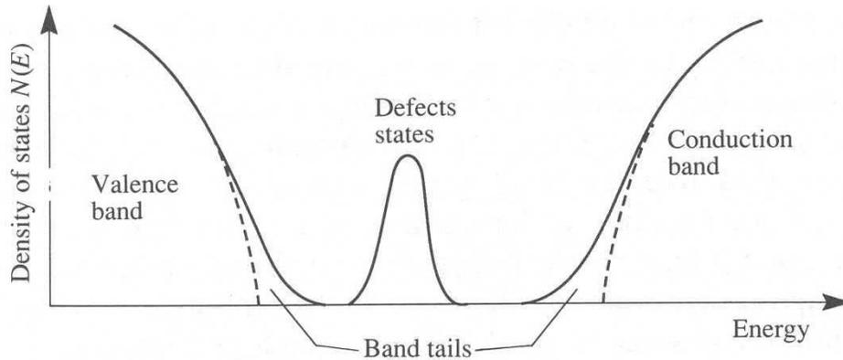
**Figure 3-4.** Schematic density of states of a-Si:H showing the localized band tails and defect states [2].
