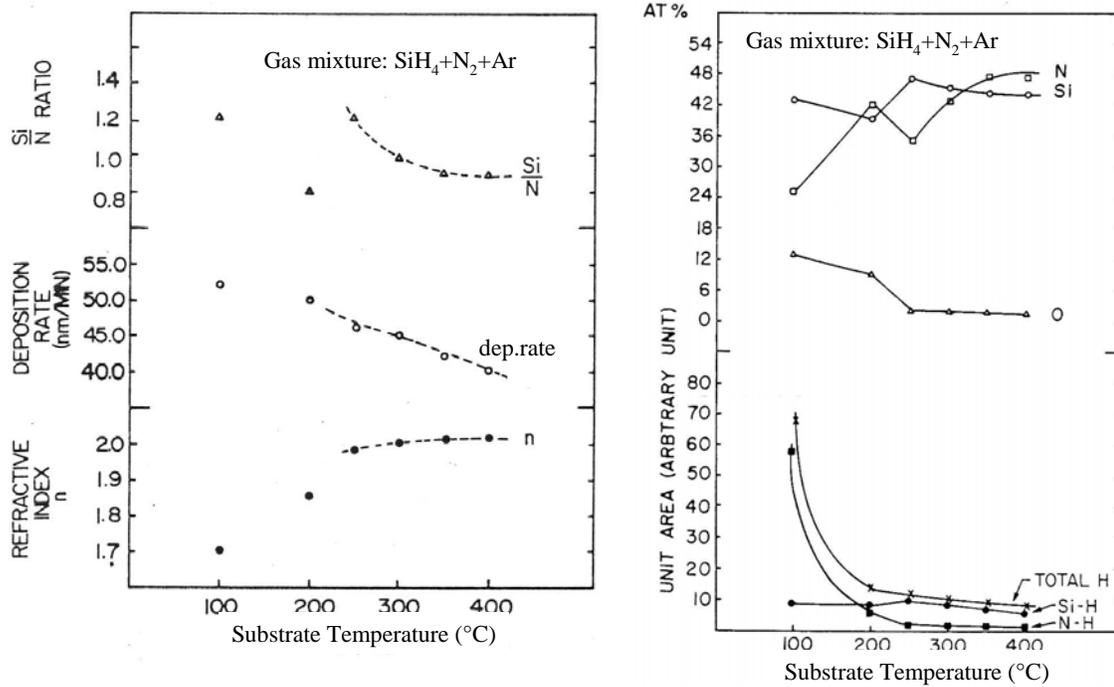
**Figure 3-8.** Dependence of SiN<sub>x</sub> properties on substrate temperature [8].
