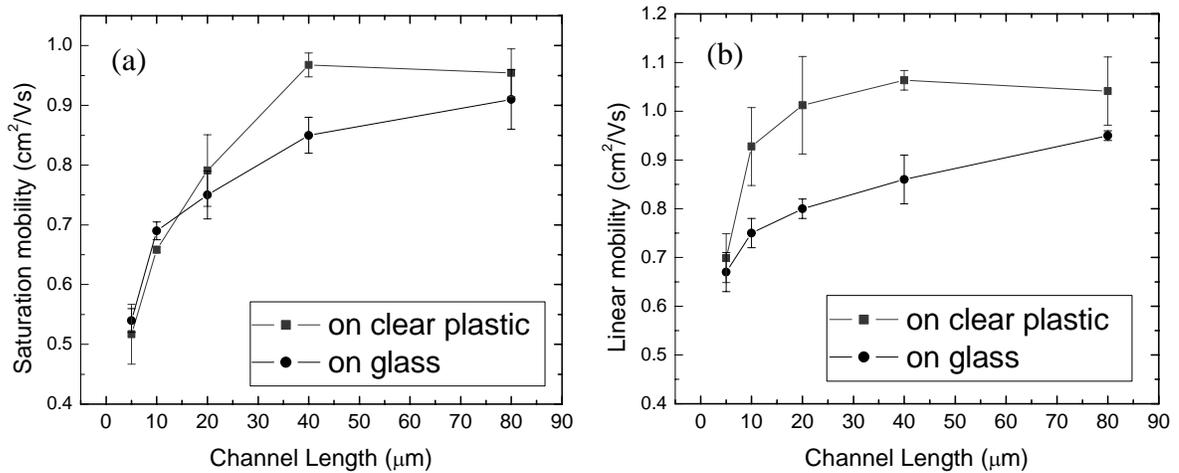
**Figure 4-11.** Mobility vs. channel length for a-Si:H TFT's fabricated at  $180^\circ\text{C}$  on clear plastic substrate and on glass, for devices with a width of  $80\mu\text{m}$ . (a) Saturation region; (b) Linear region.
