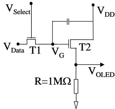
**Figure 5-7.** Schematic circuit for dynamic testing of pixels before OLED integration, with OLED replaced by a  $1\text{M}\Omega$  resistor for current monitoring.
