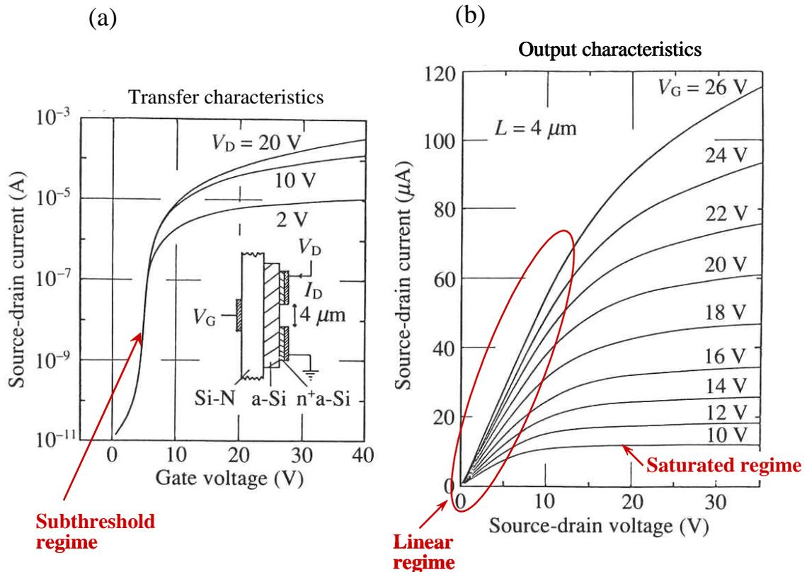
**Figure 3-9.** (a) Transfer and (b) output characteristics of an a-Si:H TFT.
