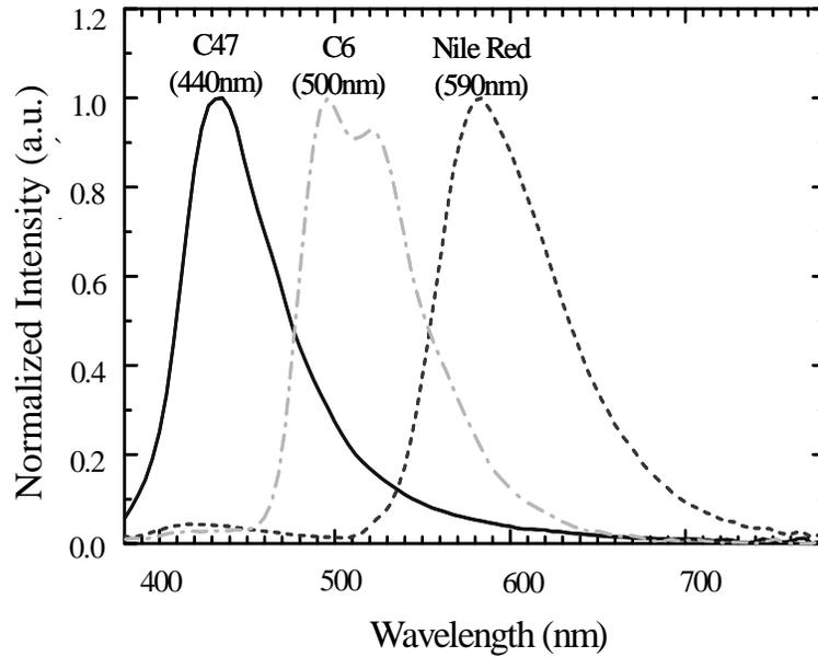
**Figure 2-22.** Electro-luminescence spectra of the red, green and blue tri-layer devices with a structure of PVK:PBD:dye (90nm)/BCP (6nm)/Alq<sub>3</sub> (40nm), with peak wavelength of 590nm, 500nm, 440nm, respectively. [29]
