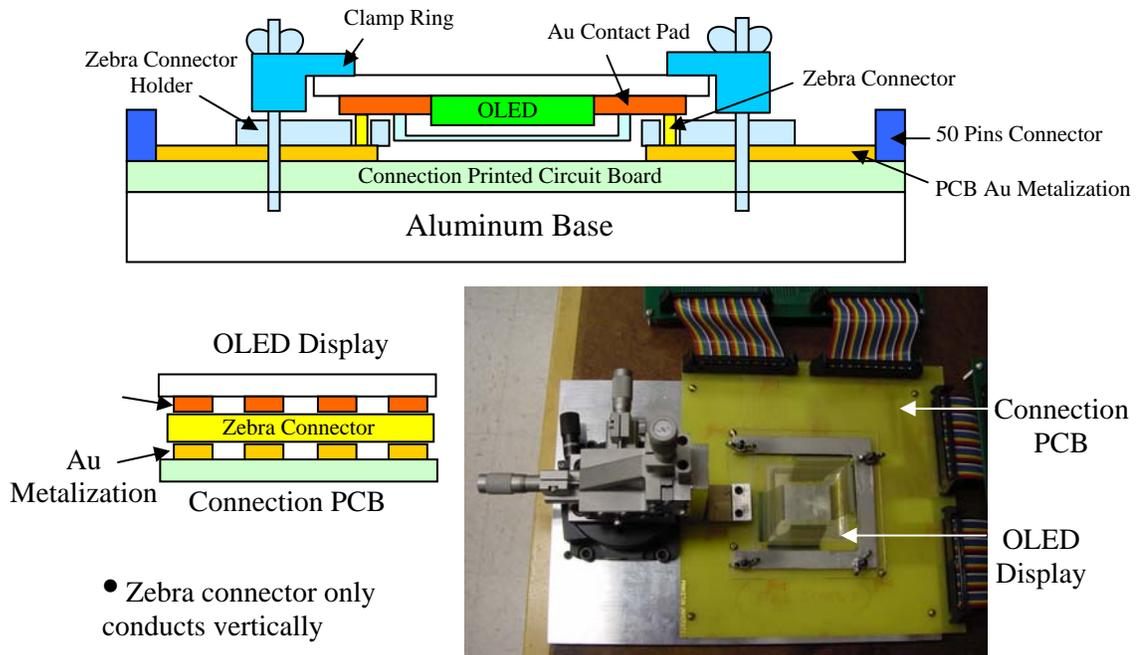
Figure A-5. Integration of the PMOLED display sample and the drivers.
