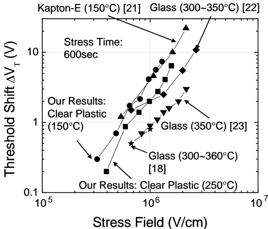
**Figure 4-19.** TFT threshold voltage shift as a function of gate electric field, held constant for 600sec. Various substrates and process temperatures are labeled. [26]
