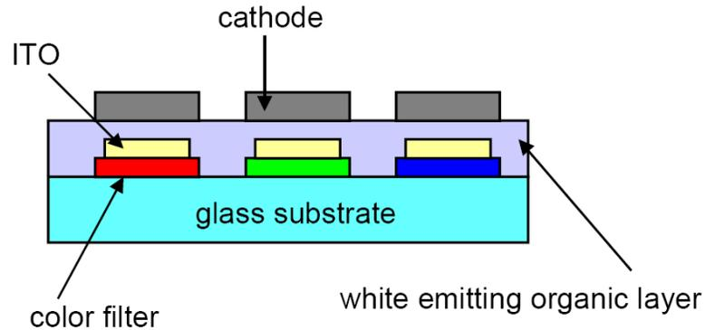
**Figure 2-3.** Red, green and blue emissions using white-emitting OLED and color filters.
