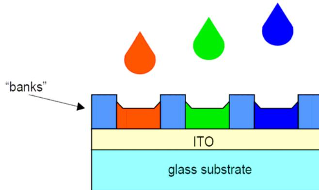
**Figure 2-1.** Ink-jet printing of red, green and blue polymer droplets onto a pre-patterned substrate with “banks” to form a more uniform polymer film.
