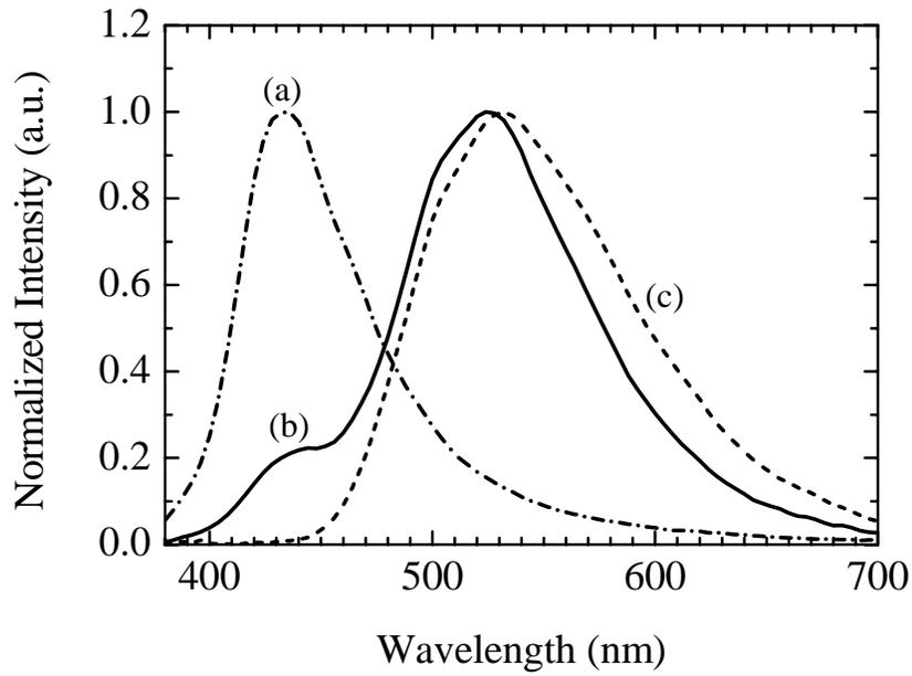
**Figure 2-17.** Normalized electro-luminescence spectra of (a) single-layer device of 90nm PVK/PBD/C47 (dash-dotted line); (b) bi-layer device of 90nm PVK/PBD/C47 + 40nm Alq<sub>3</sub> (solid line); and (c) Alq<sub>3</sub> emission reference (dashed line). [26]
