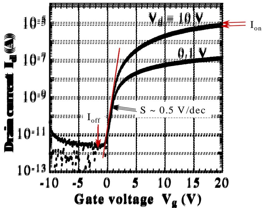
**Figure 3-12.** TFT transfer characteristics. ON current, OFF current, and sub-threshold slope are obtained from this plot.
