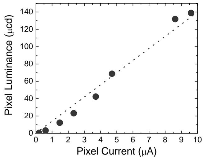
**Figure 5-14.** Pixel brightness as a function of pixel current.
