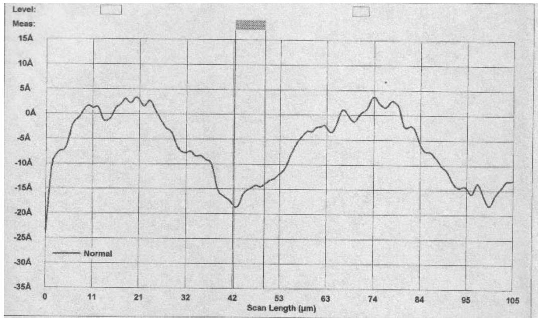
**Figure 2-10.** Surface profile of the OLED polymer. The peak-to-peak surface roughness is about 3nm.
