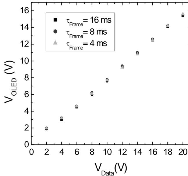
**Figure 5-9.** Stored voltage at the OLED node as a function of input data voltage for different frame times of 4ms, 8ms and 16ms.
