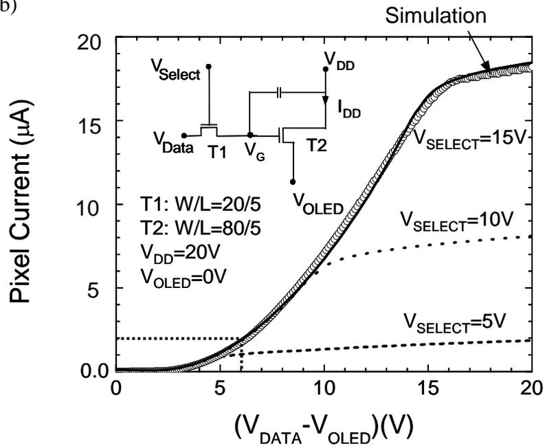
**Figure 5-6.** DC drive current as a function of data voltage tested a 2-TFT pixel before OLED integration on (a) clear plastic and (b) glass substrates for different select voltages. The open circles are simulation results using H-SPICE. The data voltage needed for 100nits display brightness ( $2 \mu\text{A}$  pixel current) is also labeled with dotted line.
