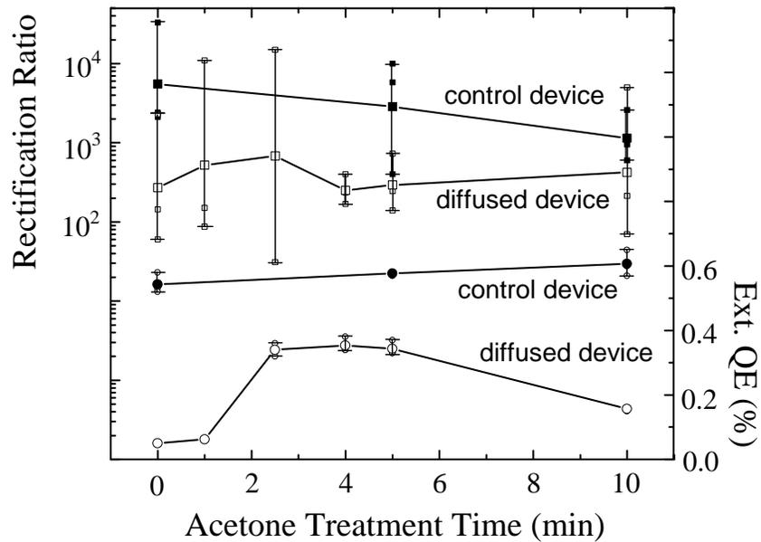
**Figure 2-14.** External quantum efficiency (circles) and the rectification ratio (squares) as a function of exposure time to acetone-vapor (partial pressure 92 torr at room temperature). Control devices (solid symbols) are devices with C6 in the spin-on solution, and diffusion devices (open symbols) are devices with transferred C6. [23]
