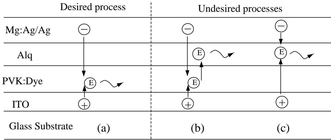
**Figure 2-18.** Emission processes in a bi-layer device. (a) Excitons formation and emission in PVK; (b) Excitons diffusion to and emit from Alq; (c) Excitons formation and emission in Alq. Motion of the electrons, holes and excitons is shown. [26]
