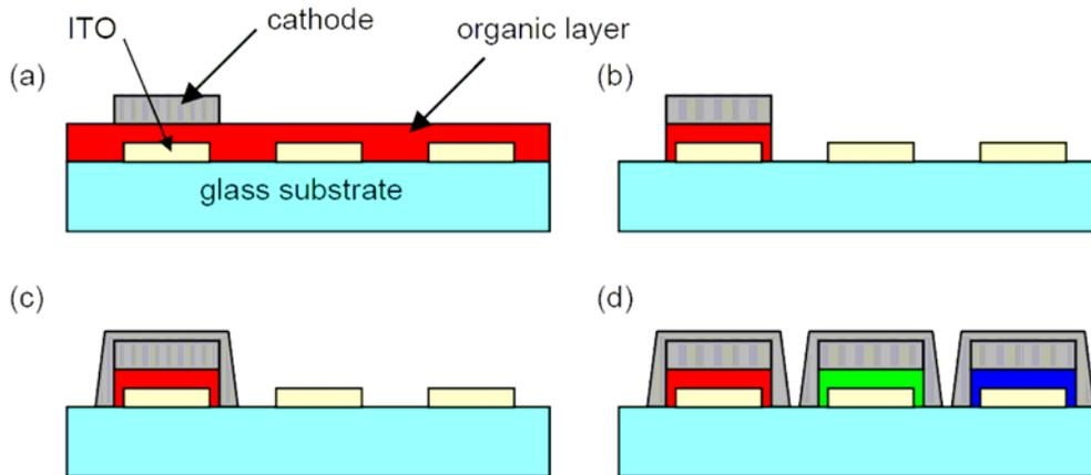
**Figure 2-2.** Fabrication of three colors by dry etching of organic layers.
