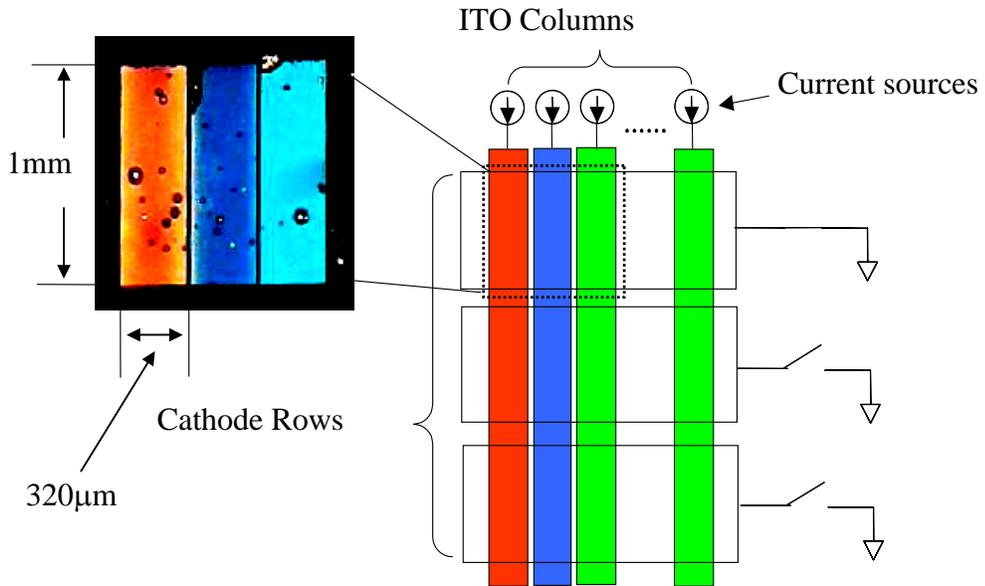
**Figure 2-26.** Electro-luminescence micrograph of a RGB pixel from a small passive matrix test array fabricated using dry-dye printing and tri-layer structure. [26]
