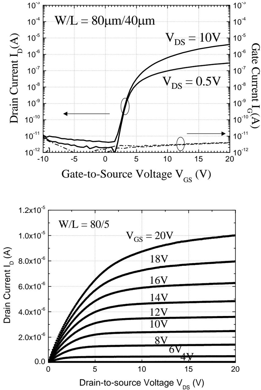
**Figure 4-13.** (a) transfer and (b) output characteristics of TFT's on free-standing clear plastic substrates, made at a maximum process temperature of 280°C.
