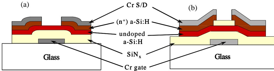
**Figure 3-5.** Schematic cross section of a-Si TFT structures: (a) back-channel etch structure; (b) etch-stop structure.
