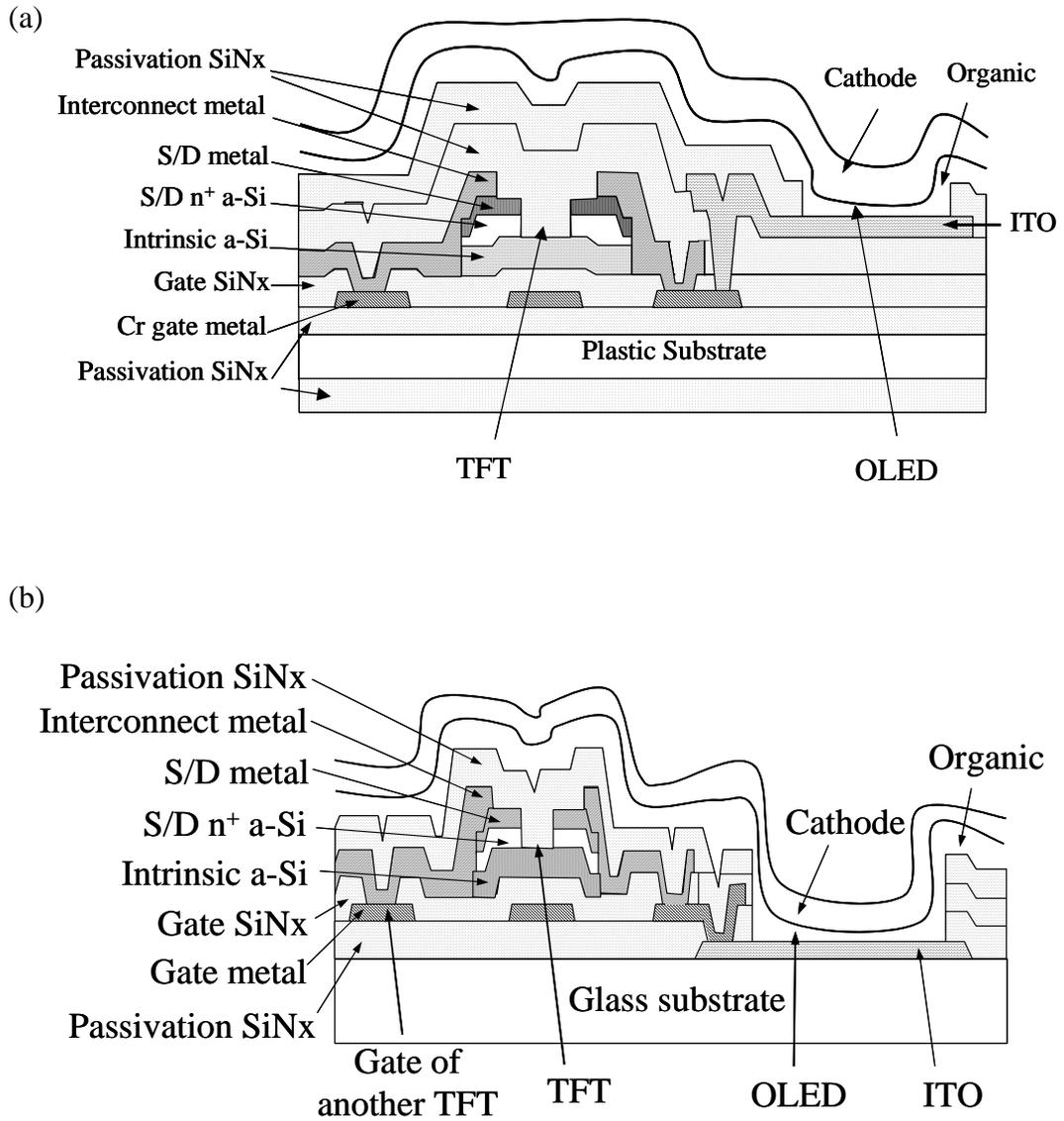
**Figure 5-4.** Schematic cross-section of the TFT-OLED integration (a) on clear plastic substrate and (b) on glass substrate.
