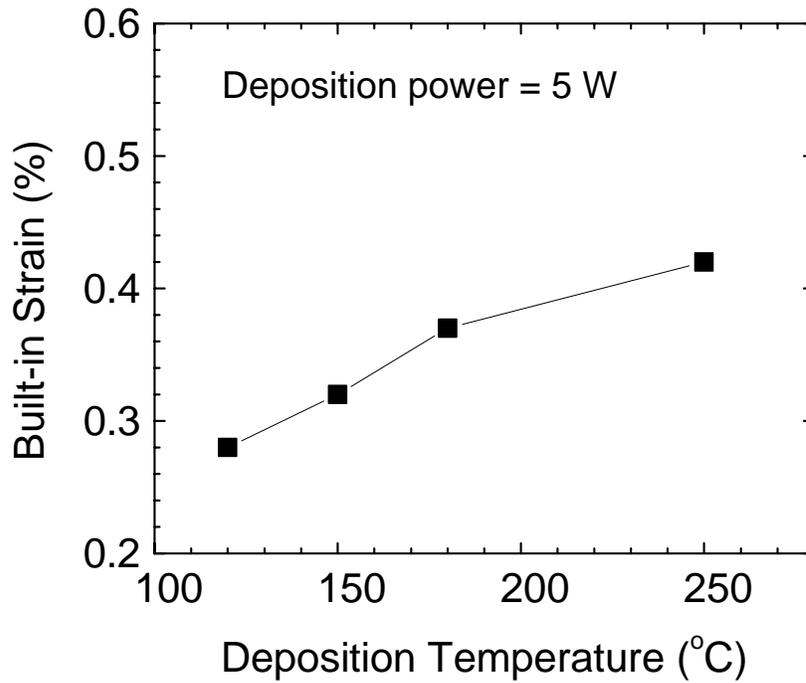
**Figure 4-4.** Built-in strain of  $\text{SiN}_x$  films deposited over a range of temperatures at 5W RF power. [25]
