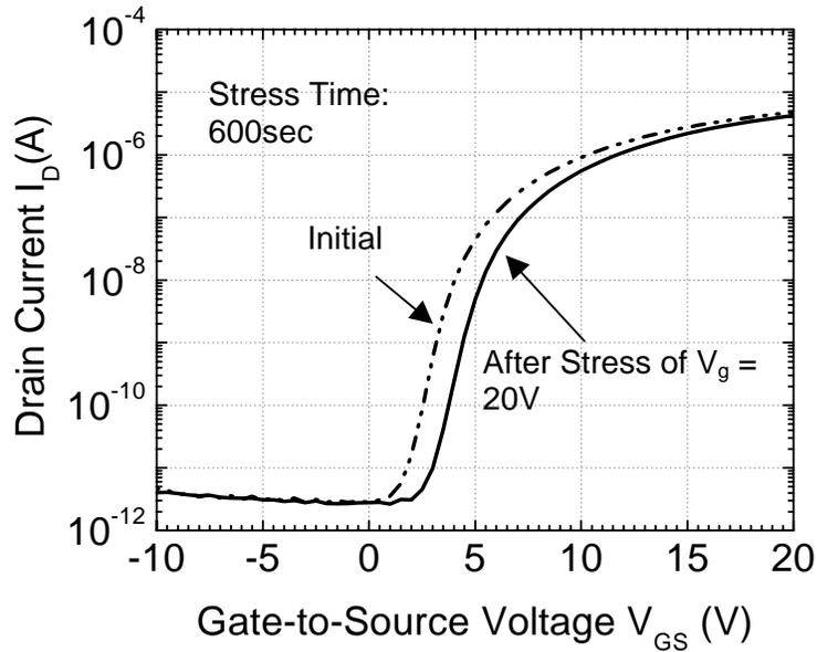
**Figure 4-15.** Transfer characteristics of a-Si TFT made at 150°C on clear plastic before (dotted line) and after (solid line) gate bias stressing at 20V for 600sec at room temperature. Size of the TFT is  $W/L = 80\mu\text{m}/20\mu\text{m}$ .
