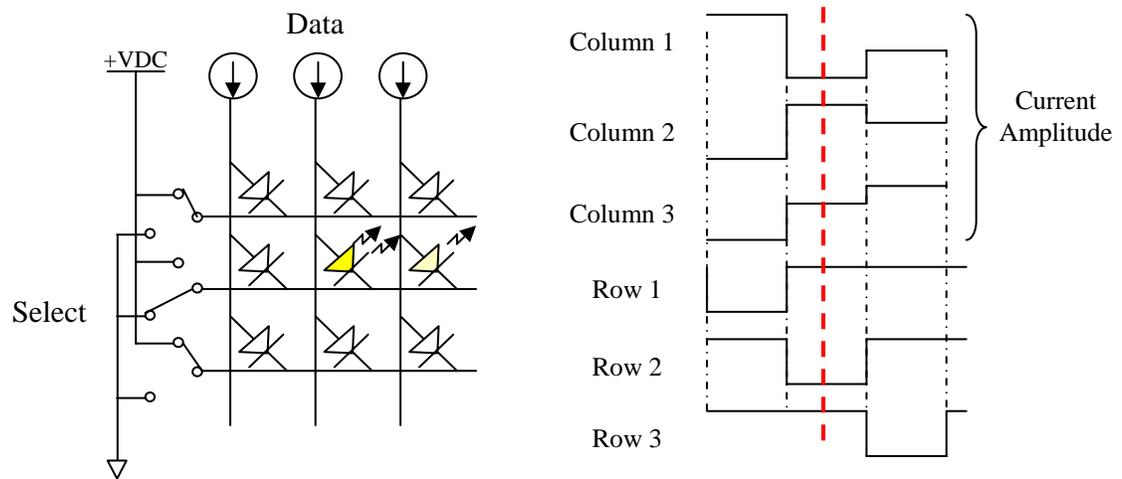
Figure A-1. Passive matrix circuit and driving waveforms.
