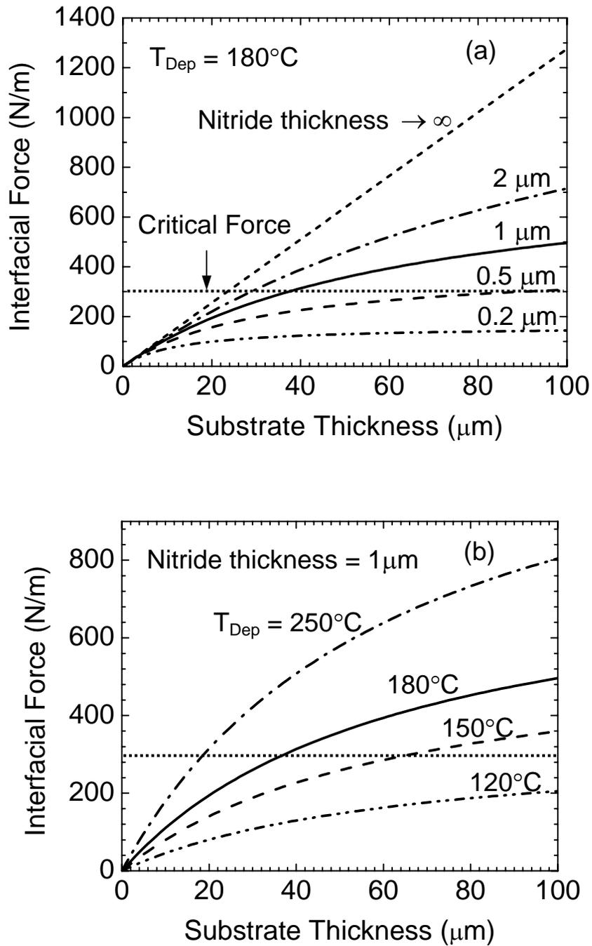
**Figure 4-6.** Calculated interfacial force as a function of substrate thickness for SiN<sub>x</sub>-on-plastic substrate A (high CTE). (a) SiN<sub>x</sub> with a range of thicknesses deposited at 180°C; (b) 1-μm-thick SiN<sub>x</sub> deposited over a range of temperatures.
