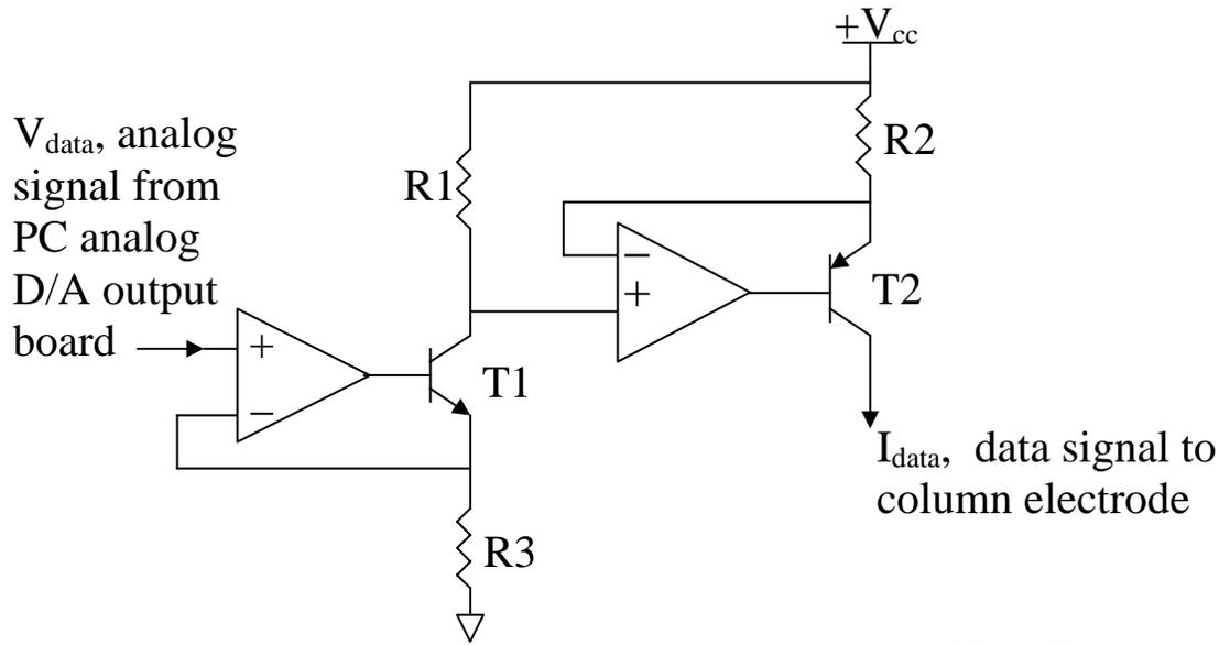
Figure A-2. Column driver: voltage controlled current source,  $I_{data} = \frac{V_{data}}{R_3} \frac{R_1}{R_2}$
