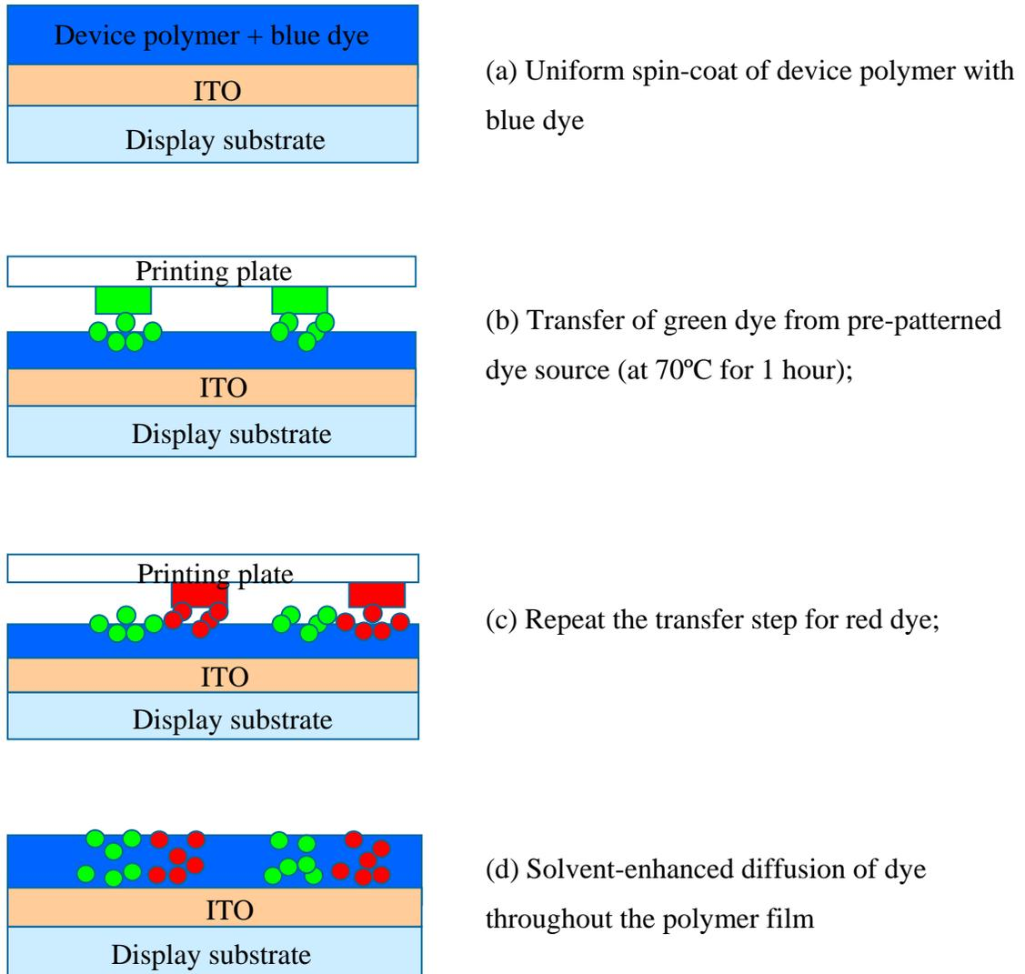
**Figure 2-6.** Schematic process flow of dry-dye printing from pre-patterned dye sources and subsequent solvent-enhanced dye diffusion for red, green, and blue patterns. Vertical dimensions are exaggerated vs. lateral dimensions.
