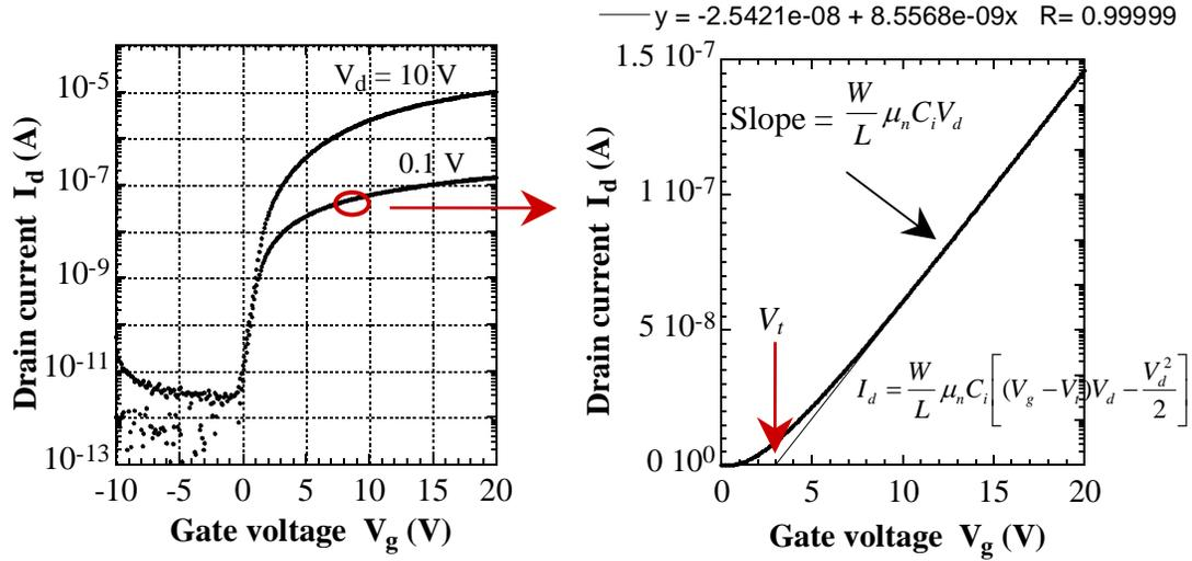
**Figure 3-10.** Drain current is plotted against gate voltage for the low drain voltage condition,  $V_d = 0.1\text{V}$ . Threshold voltage ( $V_t$ ) and linear mobility ( $\mu_n$ ) can be extracted from such a plot.
