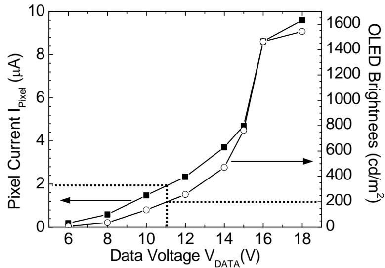
**Figure 5-13.** Measured pixel current and pixel brightness as a function of data voltage. The dotted lines indicate 11V data voltage is needed for 100 nits display brightness (assume 50% polarizer loss).
