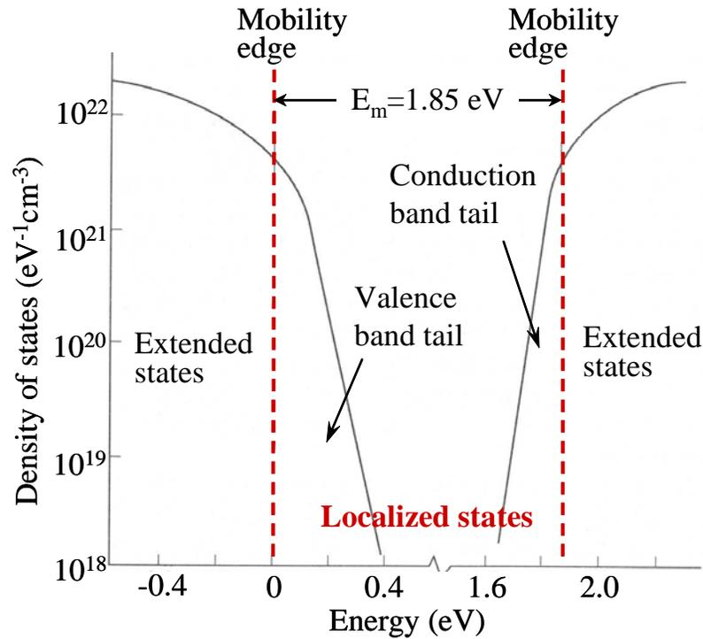
**Figure 3-3.** a-Si:H density of state as a function of energy [1]. The onset of tail states marks the edges of the mobility gap  $E_m$ .
