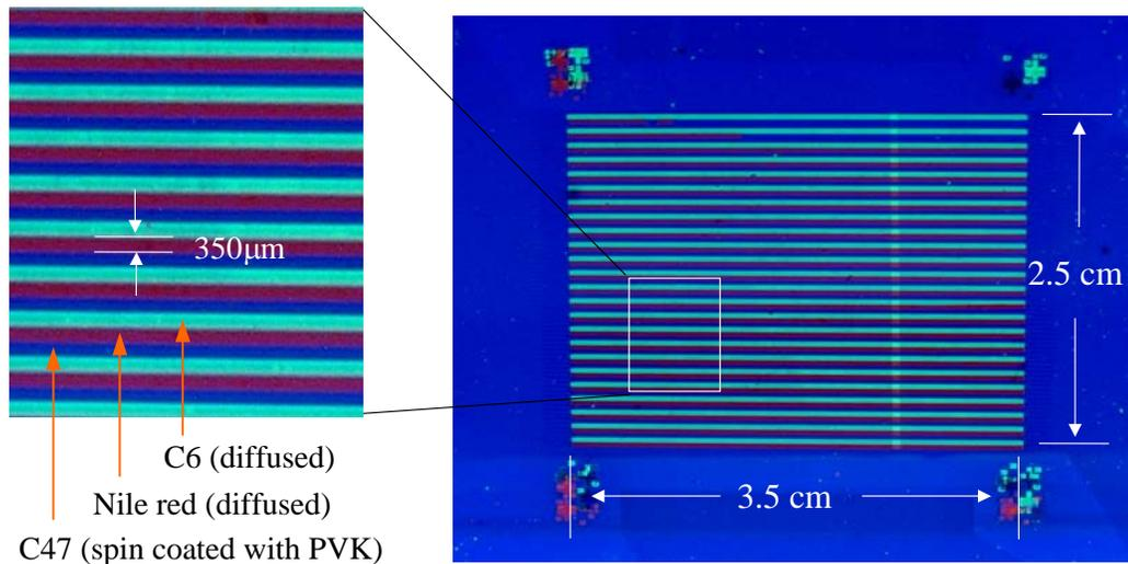
**Figure 2-12.** Photoluminescence image of a PVK/PBD/dye polymer film with 350 $\mu$ m-wide blue, green and red stripes. The blue dye C47 was spin-coated together with the polymer, and the green and red dyes C6 and NR were introduced by two printing steps and a single solvent-enhanced dye diffusion step [26].
