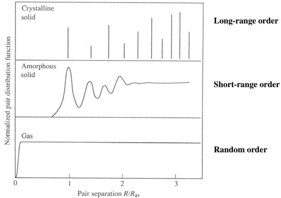
**Figure 3-2.** Normalized pair distribution as a function of separation distance [1].
