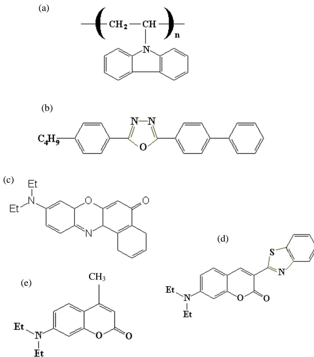
**Figure 1-2.** Chemical structure of (a) poly(9-vinylcarbazole) (PVK); (b) 2-(4-biphenyl)-5-(4-tert-butyl-phenyl)-1,3,4-oxadiazole (PBD); (c) Nile red; (d) Coumarin 6; (e) Coumarin 47.
