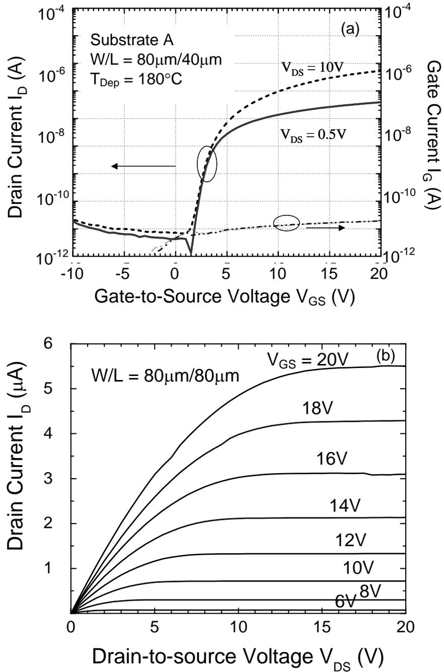
**Figure 4-10.** (a) Transfer and (b) output characteristics of TFT's processed at 180°C on clear plastic substrate A.
