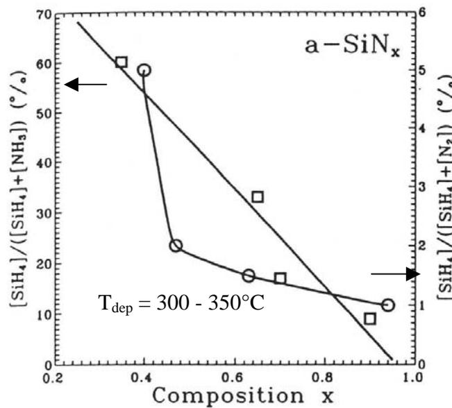
**Figure 3-7.** Dependence of  $\text{SiN}_x$  composition on the degree of  $\text{NH}_3$  or  $\text{N}_2$  dilution in the gas mixture.  $X=1.33$  is the stoichiometric composition for the best film quality [3].
