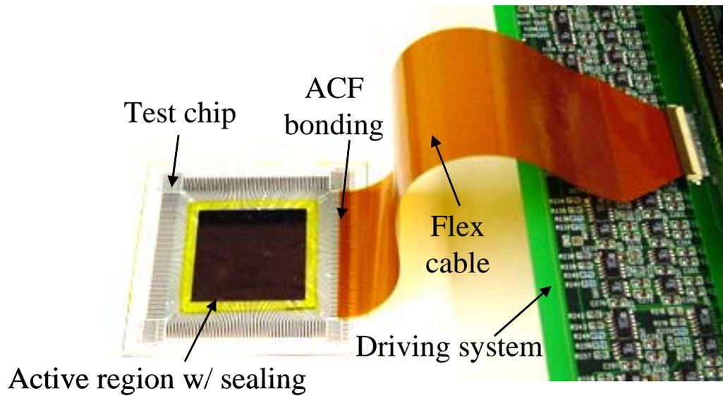
**Figure 5-10.** Picture of the finished test sample connected to driving system.
