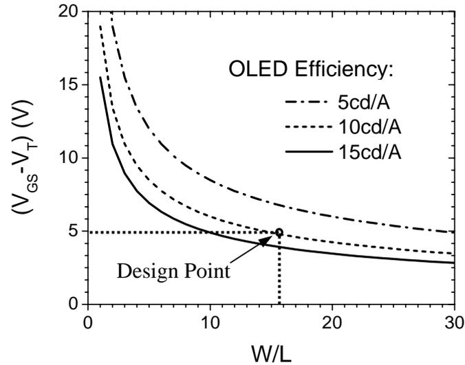
**Figure 5-2.** Required  $V_{GS} - V_T$  on drive transistor as a function of  $W/L$ , for various OLED efficiencies, assuming a pixel size of  $300\mu\text{m} \times 300\mu\text{m}$ , a polarizer efficiency of 50%, an a-Si TFT mobility of  $0.5\text{cm}^2/\text{Vs}$ , and a gate  $\text{SiN}_x$  thickness of 250nm. Our design point is  $W/L=16$ , with OLED efficiency of  $\sim 10\text{cd}/\text{A}$ .
