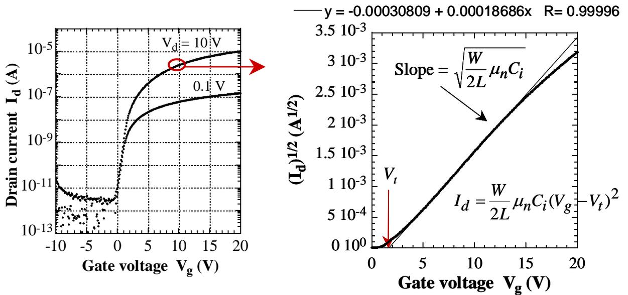
**Figure 3-11.** Drain current is plotted against gate voltage for the high drain voltage condition,  $V_d = 10V$ . Threshold voltage ( $V_t$ ) and saturation mobility ( $\mu_{n,sat}$ ) can be extracted from such a plot.
