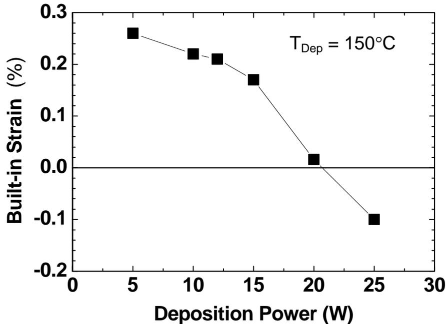
**Figure 4-3.** Built-in strain of  $\text{SiN}_x$  films deposited at  $150^\circ\text{C}$  by PECVD over a range of RF power. Low power grows films in tension (positive strain) and high power in compression (negative strain). [13]
