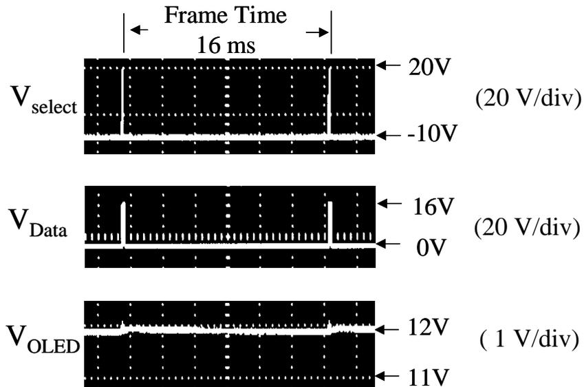
**Figure 5-8.** Applied data signal, applied select signal and  $V_{\text{OLED}}$  (proportional to drive current) vs. time shown on a multi-channel oscilloscope. The scale of each signal on the oscilloscope is also shown.
