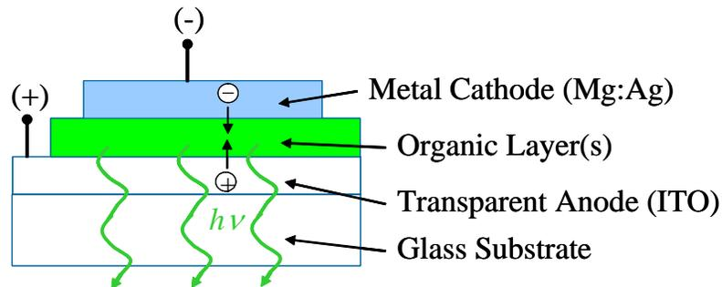
**Figure 1-1.** Schematic cross-section of an OLED
