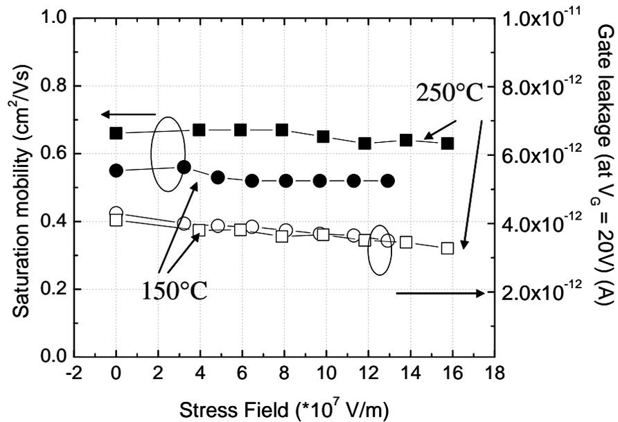
**Figure 4-17.** TFT saturation mobility (closed symbols) and gate leakage current (open symbols) after gate stressing at room temperature for 600 seconds, as a function of gate stress field. Circles are for 150°C process, squares are for 250°C process. Size of the TFT's are  $W/L = 80\mu\text{m}/20\mu\text{m}$ .
