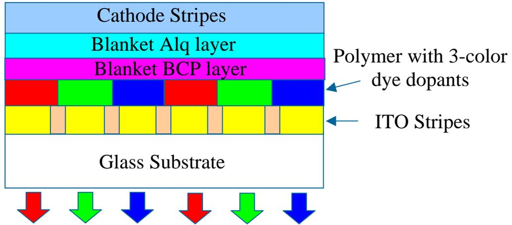
**Figure 2-25.** Schematic cross-section of the full-color passive-matrix OLED test array.
