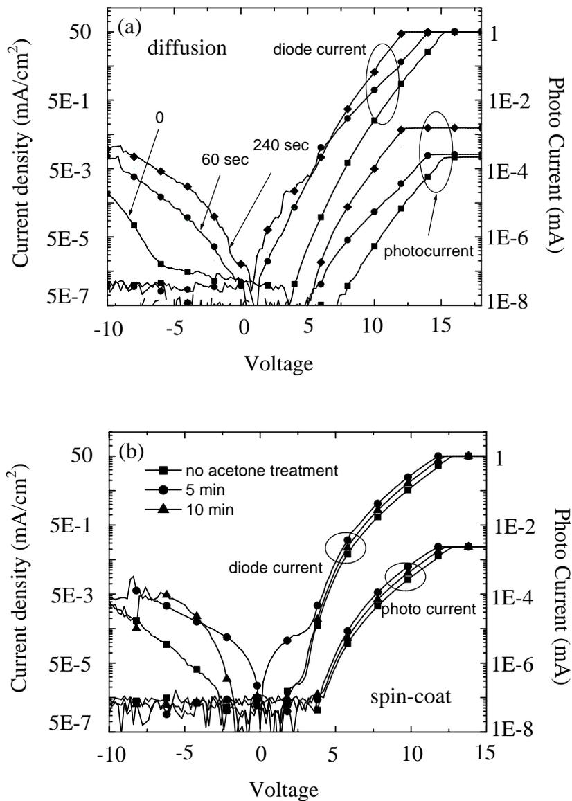
**Figure 2-13.** I-V characteristics of the PVK/PBD/C6 devices annealed in acetone-vapor (partial pressure 92 torr) for different times: (a) devices with C6 transferred from a uniform dye source of Vylon layer doped with C6 (4% by weight in the final film); and (b) control devices with C6 contained in the spin-on solution and not added by printing. [23]
