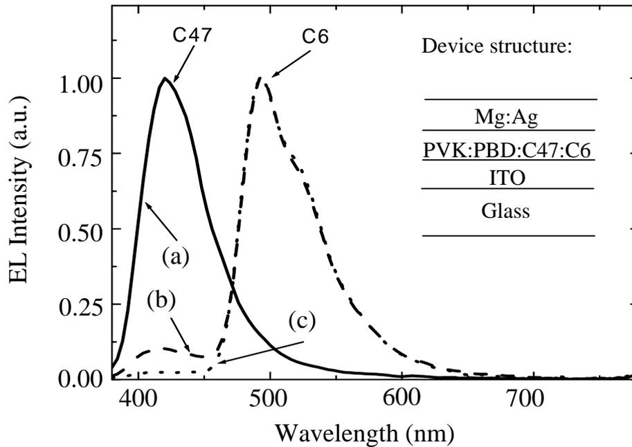
**Figure 2-11.** Electro-luminescence spectra of PVK/PBD/C47 OLED devices with C6 transferred from a dye source of Vylon layer doped with C6 (4% by weight) (a) with only the initial printing step (at 70°C for 1 hour); (b) after 60 sec of acetone-vapor annealing; and (c) after 150 sec of acetone-vapor annealing at acetone vapor pressure of 92 torr at room temperature. The inset shows the device structure [25].
