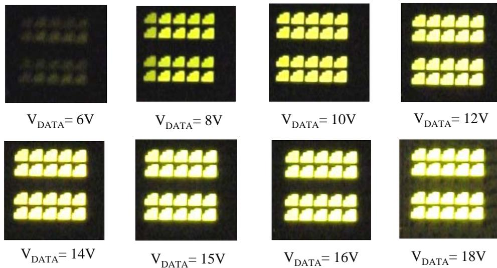
**Figure 5-11.** Images of a 5x5 AMOLED array (one row contact is missing) under QVGA driving with different data voltages.
