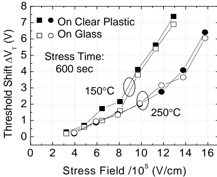
**Figure 4-16.** TFT threshold voltage shift after gate stressing at room temperature for 600 seconds, as a function of gate stress field, for clear plastic (closed symbols) and glass (open symbols) substrates. Circles are for 250°C process, squares are for 150°C process.
