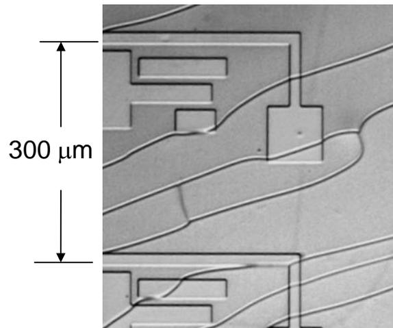
**Figure 4-9.** Cracks in device films deposited at 250°C on substrate A. Film thicknesses were: buffer nitride, 500nm; gate chromium, 100nm; gate nitride, 350nm; intrinsic a-Si, 200nm;  $\text{n}^+$  a-Si, 50nm. [25]
