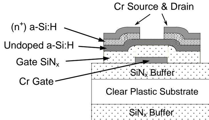
**Figure 4-8.** Schematic cross-section of the amorphous-silicon thin-film transistor structure on clear plastic substrates.[3]
