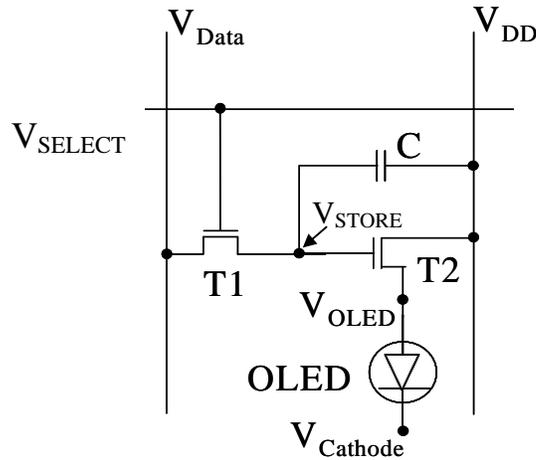
**Figure 5-1.** Schematic circuit of the 2-TFT pixel used in this work. T1 is the switching transistor, T2 the drive transistor, and C is the storage capacitor. The OLED anode is connected to source of T2.
