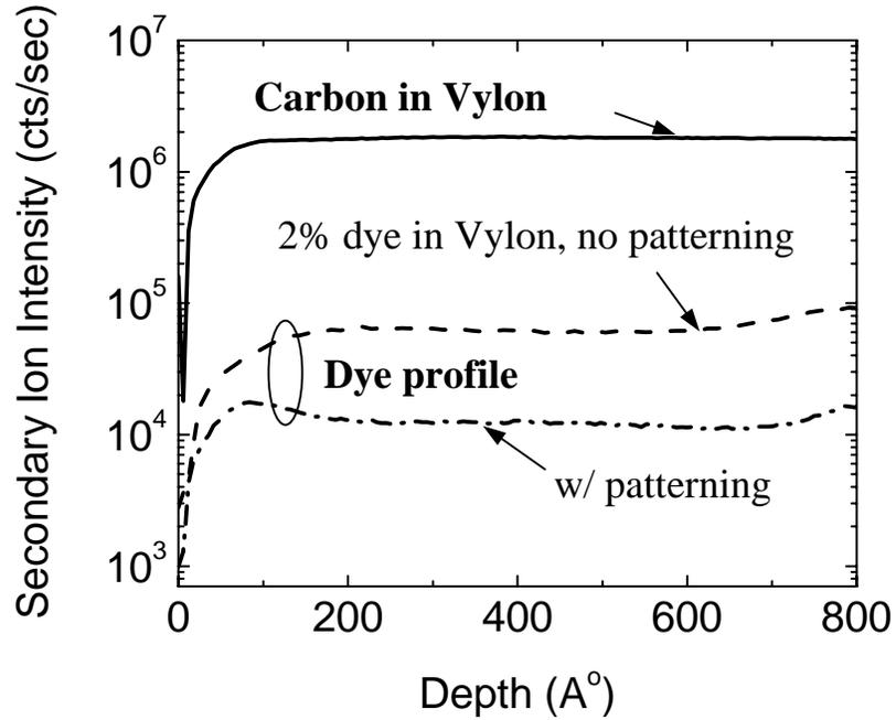
**Figure 2-23.** SIMS profiles before and after patterning of the green dye C6 doped Vylon films. [29]
