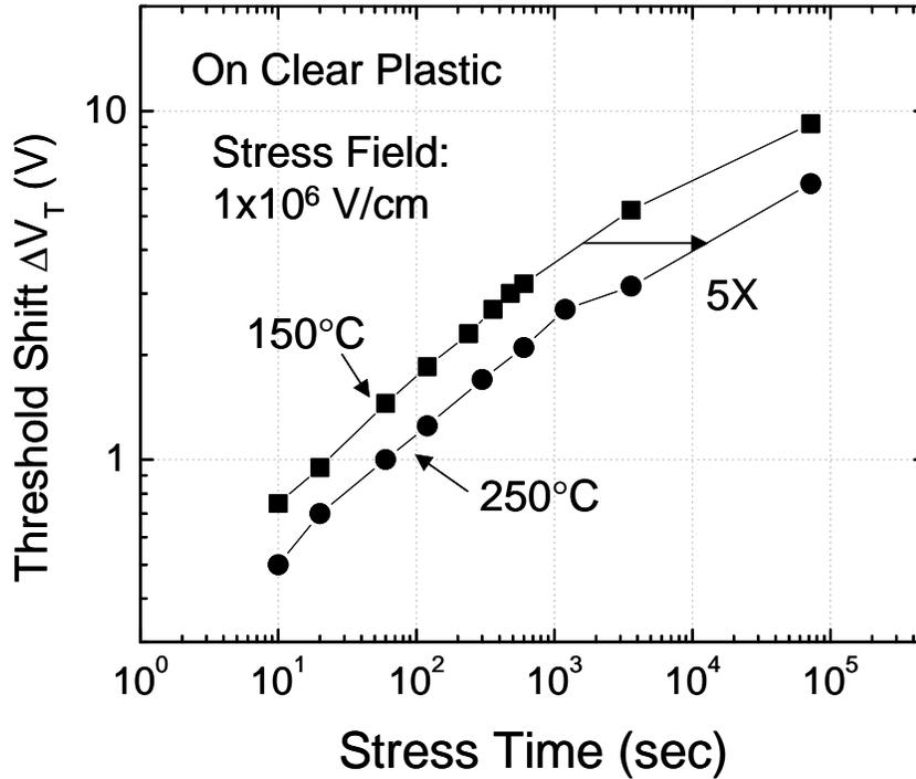
**Figure 4-18.** TFT threshold voltage shift vs. stress time at constant gate bias for TFT's made at 150°C and 250°C on clear plastic. [26]
