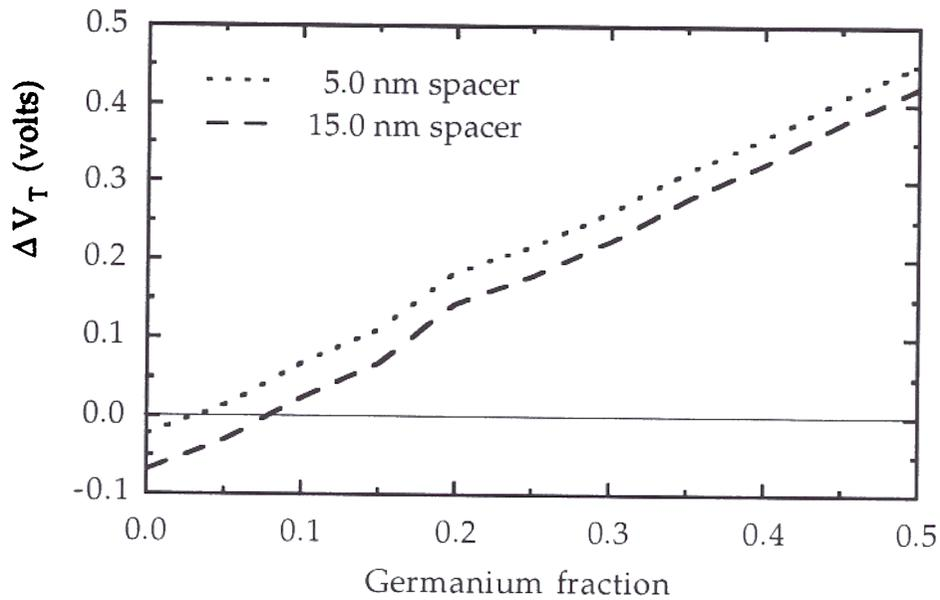
Figure 3.11 Simulated threshold voltage shift vs germanium fraction compared to a silicon MOSFET. A negative threshold shift means the  $\text{Ge}_x\text{Si}_{1-x}$  well does not form an inversion layer. Calculations for devices with a uniform doping of  $N_D = 10^{16} \text{ cm}^{-3}$ .
