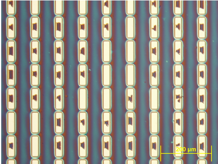
(a) Incomplete transfer, 130°C and 500 psi
