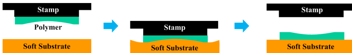
Figure 7.11: Schematic diagram of the hard-soft approach in dealing with non-flat surface.
