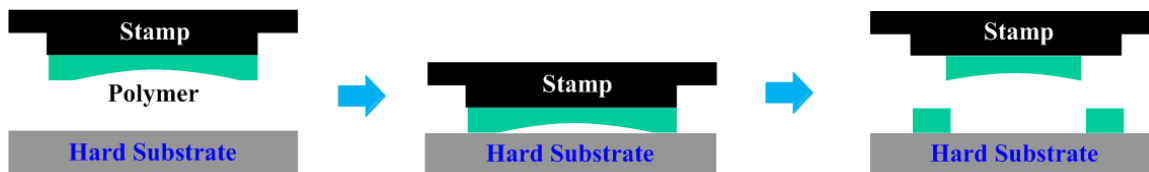
Figure 7.5: Schematic diagram of the hard-hard approach in dealing with non-flat surface.
