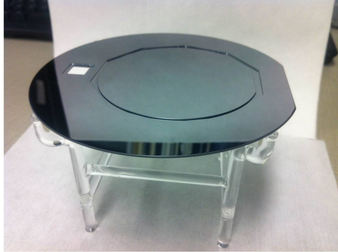
Figure C.1: The picture of a 125-mm carrier held by a 125-mm quartz wafer stand with a 75-mm wafer on it.
