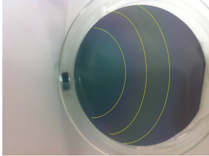
Figure C.2: The picture of 75-mm SiGe buffer carried by a 125-mm carrier wafer after a test growth. The color rings labeled by yellow lines represent the thickness nonuniformity.
