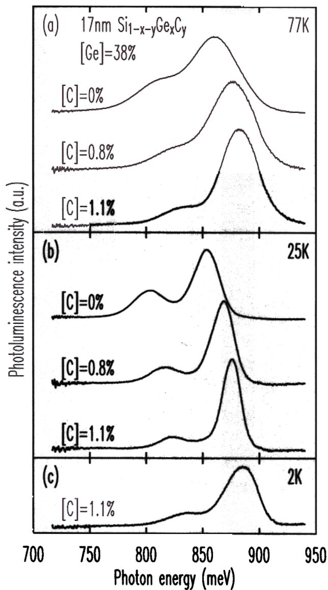
Figure 6.1: Photoluminescence spectra from  $\text{Si}_{1-x-y}\text{Ge}_x\text{C}_y$  samples with  $x = 0.38$  and various  $[\text{C}]$ . The pump power density was  $\sim 50 \text{ W/cm}^2$ . The spectra were normalized and corrected to account for the spectral response of the experimental optical path.
