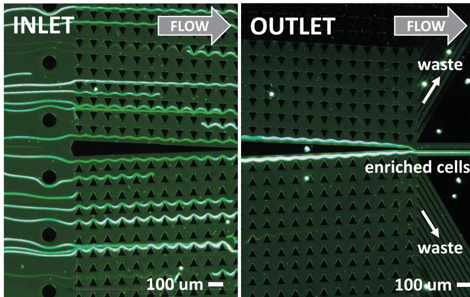
FIG. 3. **CTC enrichment in DLD array.** Trajectories of GFP-expressing MDAMB231 breast cells in an array with  $42 \mu\text{m}$  gaps,  $1/20$  array tilt, and  $7 \mu\text{m}$  critical particle size at device inlet and outlet at flow rate of  $500 \mu\text{L}/\text{min}$ . Cells are evenly dispersed at inlet but are concentrated against central wall at outlet and directed to narrow collection outlet.
