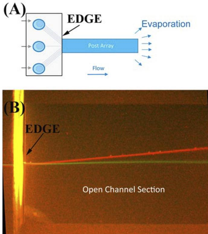
**Figure 4.** (A) Schematic of a partially sealed array. (B) Epifluorescence image of red beads ‘bumping’ at an angle to the flow direction given by the green dye jet. The flow across the device is driven by evaporation.
