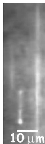
**Figure 6.** Several  $\lambda$  DNA molecules in  $100\ \text{nm}$  nanochannels. The variety of apparent lengths corresponds to different configurations of a polymer chain of finite persistence length in a channel of length less than the total polymer length. A fully stretched  $\lambda$  DNA is approximately  $16\ \mu\text{m}$  long and the right-hand side molecule is a  $\lambda$  concatamer. The scale bar corresponds to  $10\ \mu\text{m}$ .
