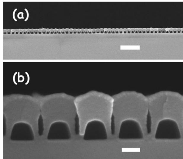
**Figure 4.** (a) Using nanoimprinting lithography nanoscale channels are uniformly defined over large areas. The scale bar corresponds to 0.5  $\mu\text{m}$ . (b) Detail of the channels resulting from nanoimprinting of PNB. The scale bar corresponds to 100 nm.
