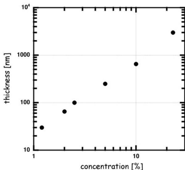
**Figure 1.** Spin curve for PNB diluted in 1, 3, 5-trimethylbenzene. The parameters are the following: 500 rpm spread during 10 s and 4500 rpm during 40 s with ramps of 100 rpm s<sup>-1</sup> and finally a solvent flash on a hotplate at 110 °C for 4 min.
