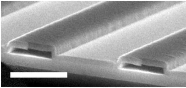
**Figure 2.** Shallow channels were made using UV lithography. 2.5% PNB was spun at 4500 rpm to achieve a 100 nm thickness. The scale bar corresponds to 1  $\mu\text{m}$ .
