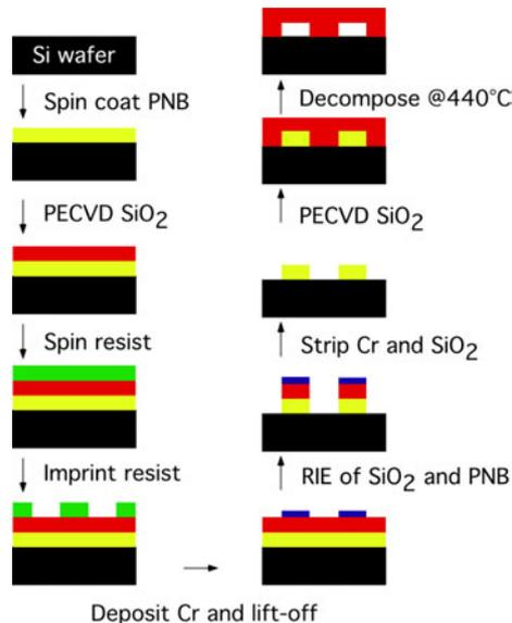
**Figure 3.** The process steps used for making nanochannels based on nanoimprinting of PNB.
