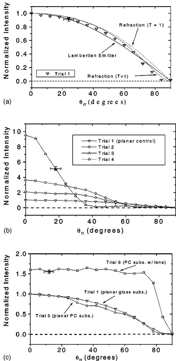
FIG. 2. (a) Measured far-field intensity distribution pattern for planar glass substrate and the expected profiles of a Lambertian emitter, and the  $T=1$  [Eq. (4)] and  $T \neq 1$  refraction models. (b) Experimental results for glass substrate devices with and without lenses. (c) Experimental results for PC substrate devices with and without lenses, along with the planar glass substrate results.
