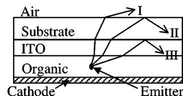
FIG. 1. Ray diagrams in planar OLEDs demonstrating loss by light trapping in the substrate (ray II) and in the organic/anode layers (ray III). Only light emitted at sufficiently small angles will escape (ray I).
