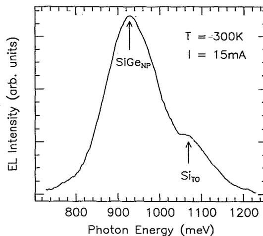
FIG. 3. Electroluminescence spectra with room temperature heat sink with 15 mA drive current.
