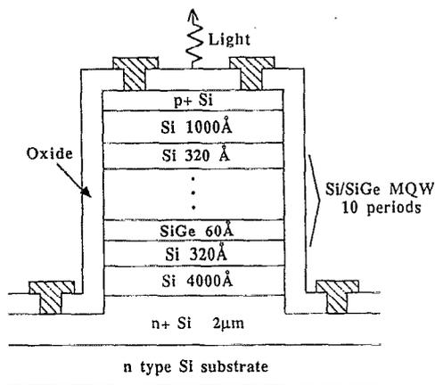
FIG. 1. Device schematic. The active regions consists of ten layers of Si—320 Å/Si<sub>0.65</sub>Ge<sub>0.35</sub>—60 Å.
