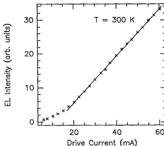
FIG. 4. Peak intensity of 1.3 μm emission with room temperature heat sink vs drive current.
