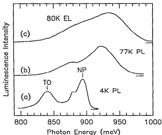
FIG. 2. Photoluminescence spectra at (a) 4.2 K and (b) 77 K, and (c) electroluminescence spectrum with 10 mA drive current and heat sink temperature at 80 K.
