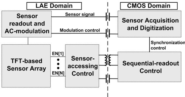
Fig. 11. Architectural blocks of the sensing subsystem.
