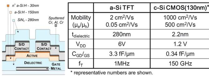
Fig. 3. Structure of the a-Si TFTs fabricated in-house and a summary of their electrical characteristics.
