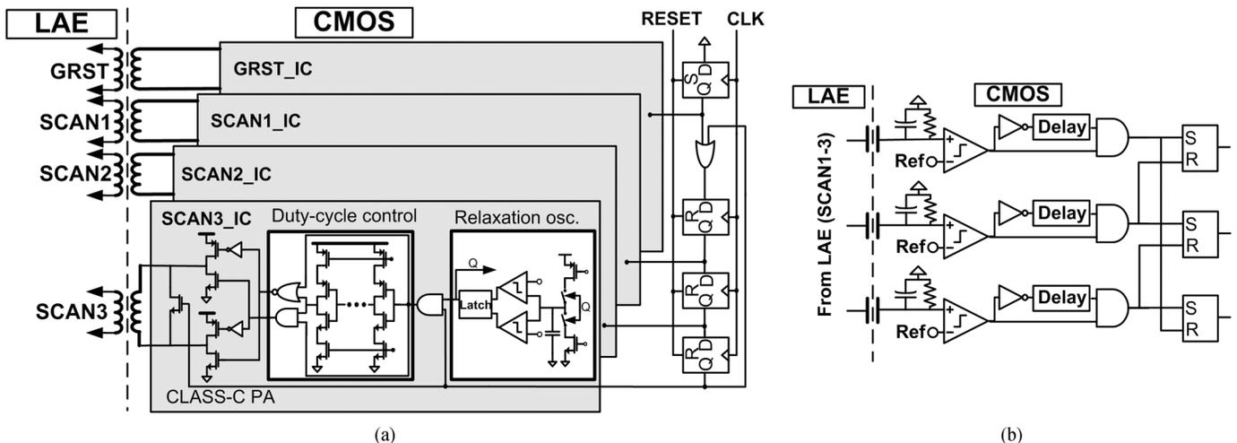
Fig. 18. Sequential readout control block for (a) IC-based sensor-accessing control and (b) LAE-based sensor-accessing control.
