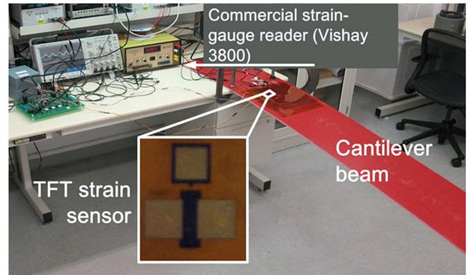
Fig. 22. Testing setup used in the lab for the sensing subsystem.
