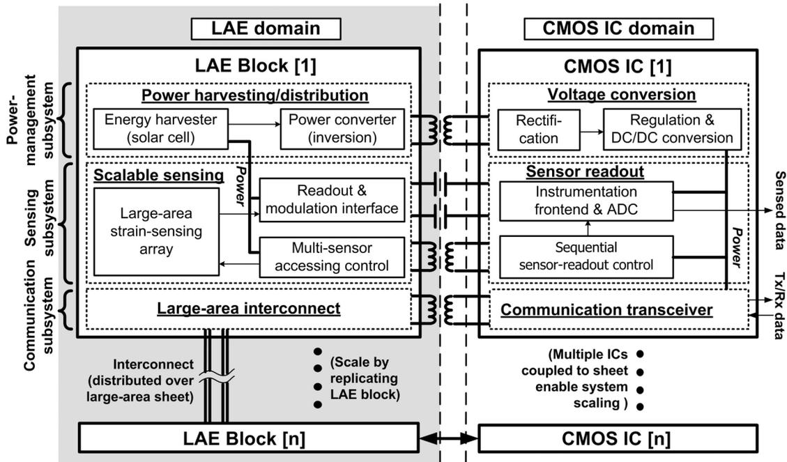
Fig. 1. Hybrid LAE-CMOS system architecture, showing functionality partitioning enabled by non-contact interfaces.
