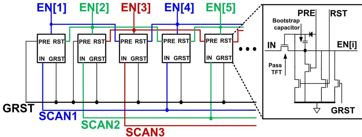
Fig. 14. Thin-film scanning circuit for generating sequential TFT-sensor enable signals ( $EN[i]$ ) using four input control signals (GRST, SCAN1–3).
