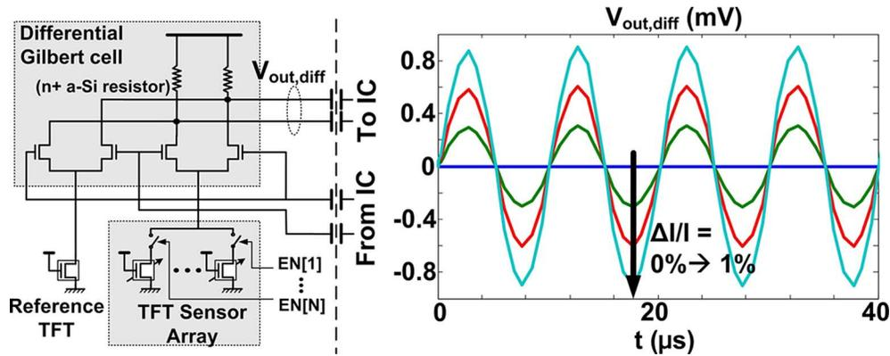
Fig. 13. Thin-film differential Gilbert cell with simulations showing the output voltage generated due to different  $\Delta I_{DS}/I_{DS}$  from the TFT sensors.
