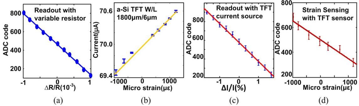
Fig. 23. Sensor subsystem response showing (a) CMOS acquisition characterization with a variable resistor driven by the CMOS-generated modulation signal, (b) isolated strain response of TFT-sensor current, (c) isolated readout performance of acquisition circuits obtained by using a calibrated TFT current source at the tail node of the LAE Gilbert cell, and (d) overall strain response of the system using TFT sensors.
