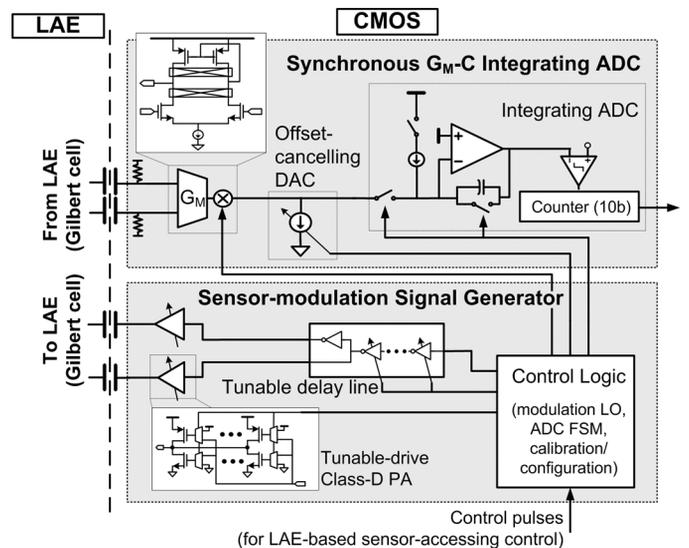
Fig. 17. Details of the CMOS  $G_M$ -C integrating ADC and sensor-modulation signal generator.
