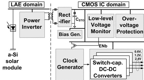
Fig. 4. Architectural blocks of the power-management subsystem.
