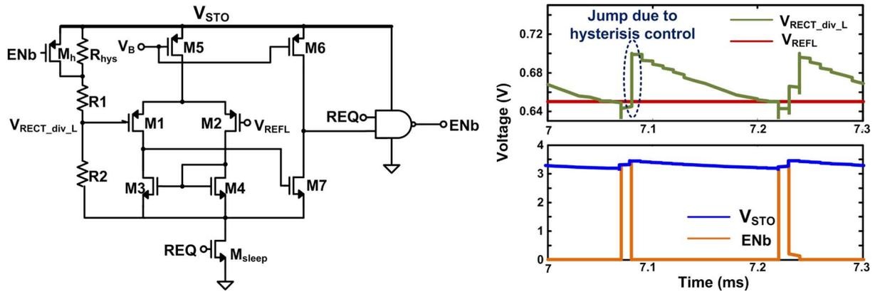
Fig. 7. Circuit details of low-level voltage monitor and its simulated waveforms.
