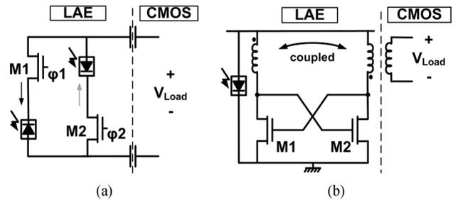
Fig. 5. TFT power inverters based on (a) Class-D topology and (b) LC-power-oscillator topology.
