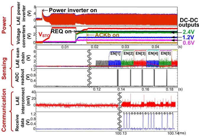
Fig. 20. Measured waveforms for system prototype from oscilloscope capture.
