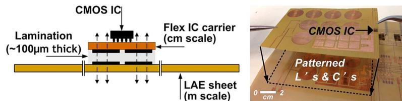
Fig. 2. Non-contact interfaces for scalable system assembly achieved via sheet lamination of a flexible IC carrier on the large-area sheet.
