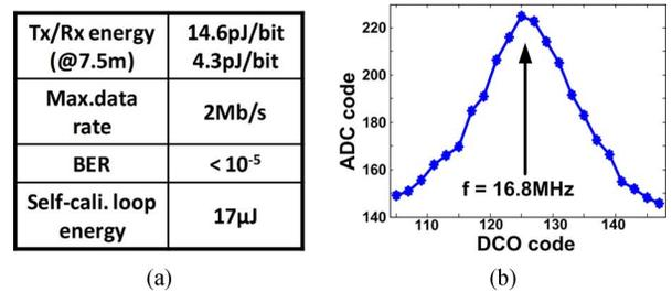
Fig. 24. Communication subsystem measurements, showing (a) the performance summary [7], and (b) calibration-loop sweep used to set the DCO frequency to the interconnect resonant point.
