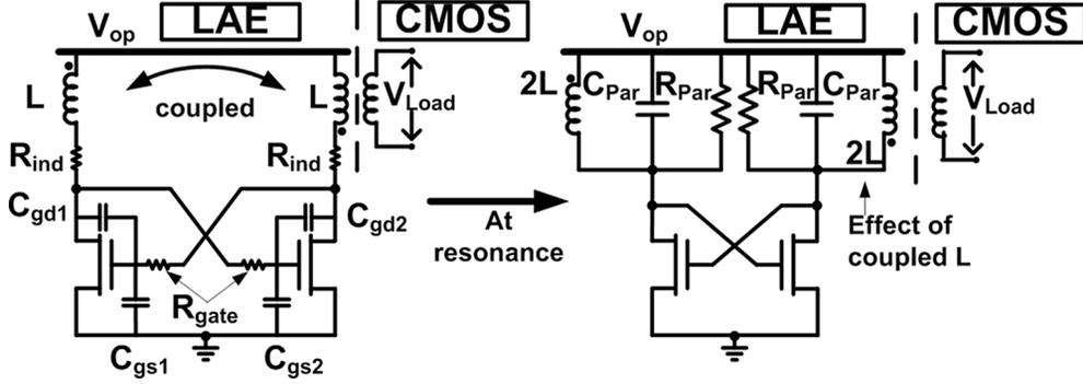
Fig. 6. LC-oscillator analysis considering the TFT parasitics.
