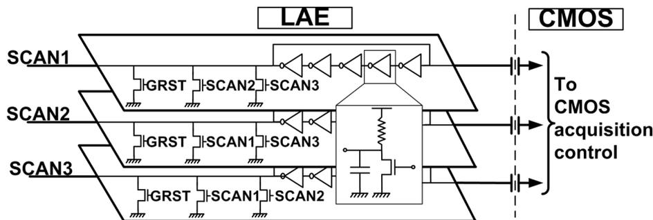
Fig. 16. LAE-based three-phase control is achieved using NOR-gate coupled TFT oscillators and interfacing with IC is achieved capacitively to enable edge detection for synchronization.
