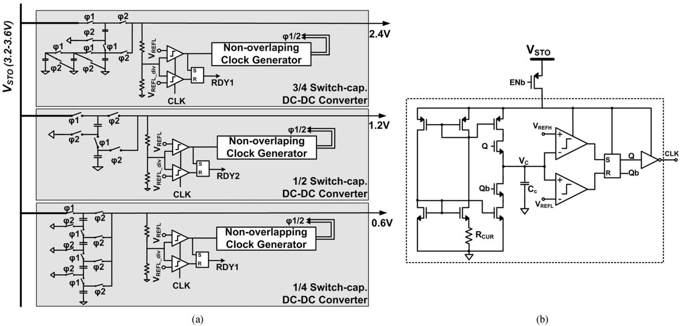
Fig. 10. (a) Details of three DC/DC converters for 0.6 V, 1.2 V and 2.4 V supplies. (b) Relaxation oscillator circuit for DC/DC converter clock generation.
