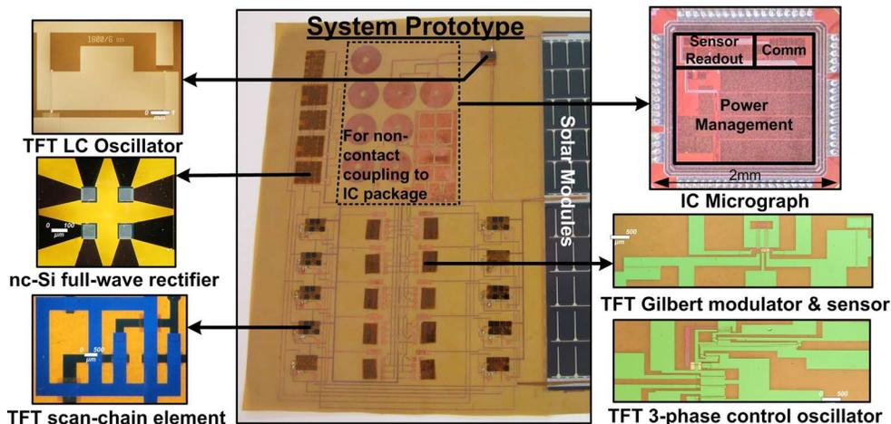
Fig. 19. System prototype, consisting of CMOS IC fabricated in a 130 nm process from IBM and LAE circuits fabricated in house on 50- $\mu\text{m}$ -thick polyimide.
