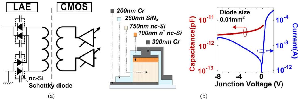
Fig. 15. IC-based sensor-accessing control uses (a) a thin-film full-wave rectifier based on Schottky diodes for demodulation of IC control signals, and (b) nanocrystalline silicon (nc-Si) diodes yield  $1000\times$  higher current density (compared to a-Si diodes), enabling smaller devices and reduced resonant capacitance for higher frequency of the inductive interfaces.
