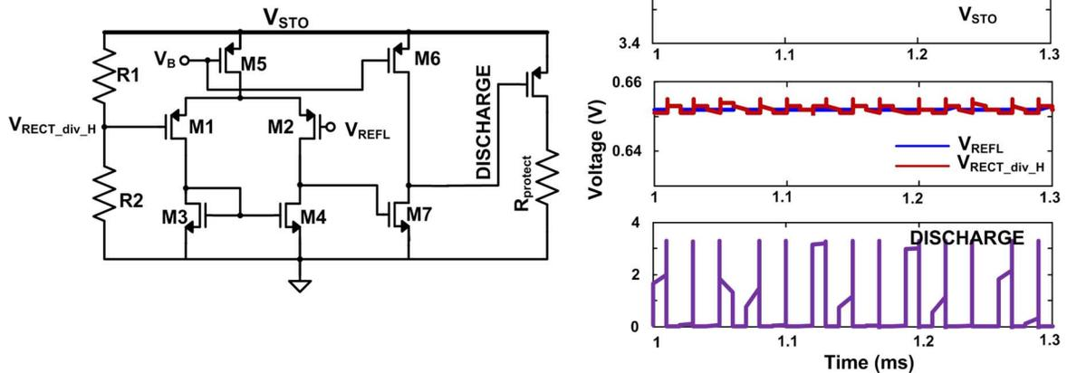
Fig. 8. Details of the over-voltage protection circuit and its simulated waveforms.
