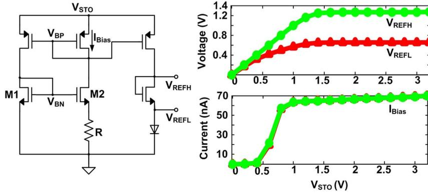
Fig. 9. Sample biasing and reference-generation circuit with DC sweep on  $V_{STO}$  showing the generation of biasing levels ( $V_{REFH}/V_{REFL}$ ) for the low-level voltage monitor, over-voltage protection circuit, DC-DC converters, and clock generator.
