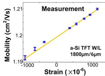
Fig. 12. Mobility response of TFT-based strain sensors.
