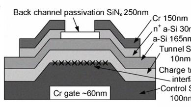
Figure 2. Structure of the a-Si Si<sub>x</sub> Trap TFT (ST-TFT) memory. Charge trapping medium is a layer of defects formed by RIE. Since the charge traps do not form a conductor, the overlapping regions between the S/D and the charge trapping layer do not contribute to parasitic capacitance that affect device behavior.
