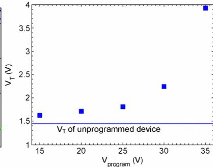
Figure 5. Programming characteristics of the ST-TFT. Devices are programmed with S/D grounded, and  $V_{program}$  applied to the gate for 10ms.
