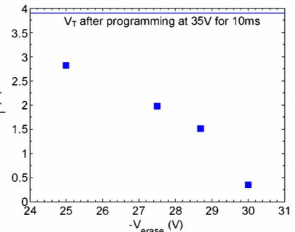
Figure 6. Erasing characteristics of the ST-TFT. Devices are first programmed with S/D grounded, and 35V applied to the gate for 10ms. Then erased by applying  $V_{erase}$  to the gate for 10ms with the S/D grounded.
