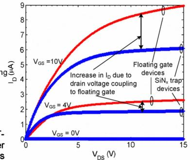
Figure 3.  $I_{DS}$  vs  $V_{DS}$  for an FG-TFT and a ST-TFT fabricated on the same wafer with the same W/L (60/5) and gate dielectric thickness (270nm).
