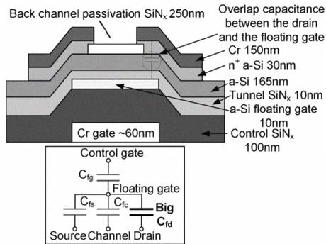
Figure 1. Structure of the a-Si floating gate TFT (FG-TFT) memory. Large overlap between FG and drain results in strong capacitive coupling.
