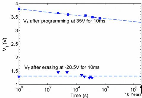
Figure 7. The room-temperature retention characteristics of the ST-TFT. Devices are programmed/erased and stored at room temperature with all electrodes floating. The shown dotted lines are extrapolations of measured data points (solid squares and triangles).
