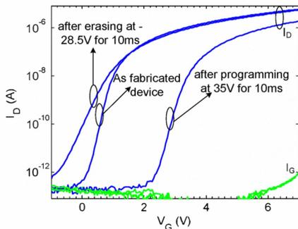
Figure 4. DC transfer characteristics ( $V_{DS} = 8V$  and  $V_G$  swept from 7 to  $-1V$  in 50mV increments) of the ST-TFT at various stages of the program/erase cycle. Program:  $V_G$  held at 35V for 10ms with S/D grounded. Erase:  $V_G$  held at  $-28.5V$  for 10ms with S/D grounded
