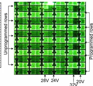
Figure 9. 10x10 AMOLED display driven with  $V_{data} = 8V$  and  $V_{DD} = 10V$ . The odd rows have unprogrammed pixels. The even rows have programmed pixels. Within each programmed row, the pixels are programmed to 4 intensity levels as indicated by the arrows. Note that the entire display is driven with a single DC data voltage. No pixel refreshes are being performed. The image remains the same after display powers off and on again.
