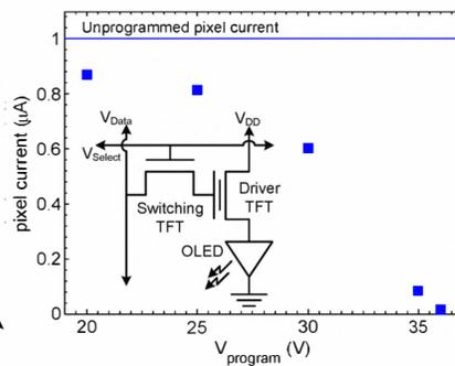
Figure 8. Current through the driver TFT after pixel programming. Inset shows the circuit schematic of an AMOLED pixel with integrated ST-TFT memory. Note the absence of the storage capacitor that is common in conventional AMOLED pixels. Pixels are first programmed by applying  $V_{program}$  to the data line for 10ms, with  $V_{DD}$  electrode grounded the select line high. Pixel currents are then measured with  $V_{data} = 8V$  and  $V_{DD} = 10V$ .
