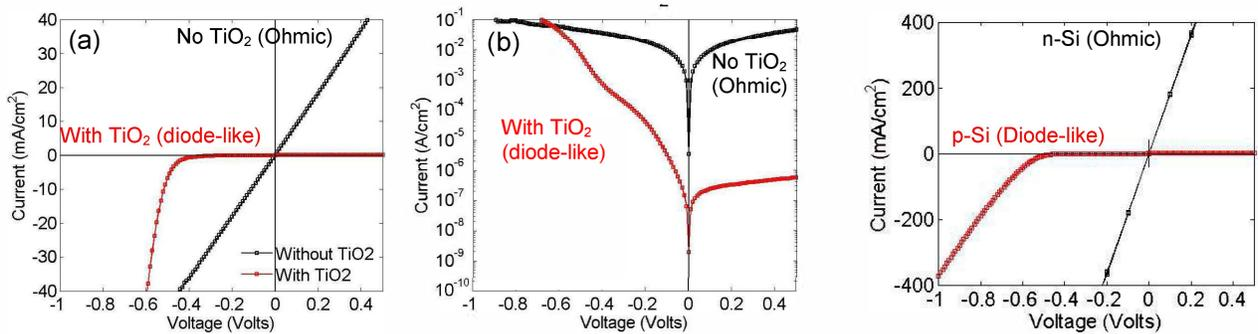
**Fig. 2:** The dark I-V characteristics of Al/TiO<sub>2</sub>/p-Si heterojunction diode compared to Al/p-Si Schottky diode on a (a) linear and (b) semilog scale. Without TiO<sub>2</sub> the junction is ohmic but with TiO<sub>2</sub> the junction is rectifying, indicating that the TiO<sub>2</sub>/Si junction blocks holes ( $\Delta E_V \gg 0$  eV).
