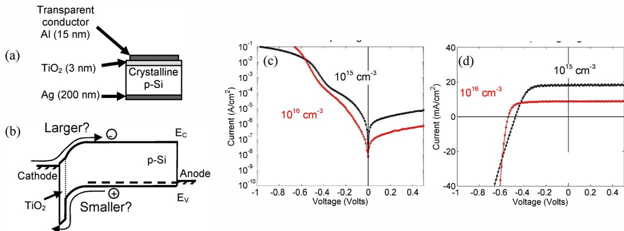
**Fig. 4:** (a) Structure of the TiO<sub>2</sub>/pSi heterojunction solar cell (b) band-diagram of the solar cell, in dark and under forward-bias, showing the hole and electron currents. The I-V characteristics for  $10^{15}$  and  $10^{16}$  cm<sup>-3</sup> doped Si wafers (c) in dark and (d) under 200 mW/cm<sup>2</sup> halogen lamp illumination. The variation in short-circuit current is probably due to unintended variation in the thickness of the Al electrode.
