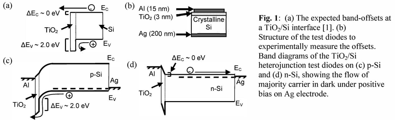
**Fig. 1:** (a) The expected band-offsets at a TiO<sub>2</sub>/Si interface [1]. (b) Structure of the test diodes to experimentally measure the offsets. Band diagrams of the TiO<sub>2</sub>/Si heterojunction test diodes on (c) p-Si and (d) n-Si, showing the flow of majority carrier in dark under positive bias on Ag electrode.
