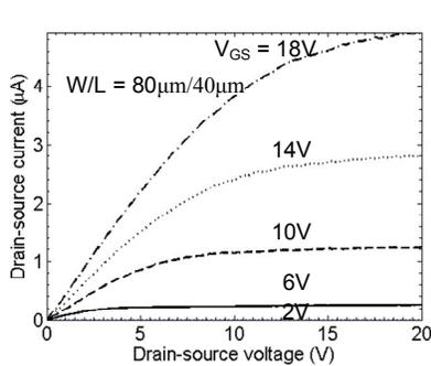
Fig. 3. Room-temperature output characteristics of a top gate a-Si TFT with self-aligned silicide source drains.
