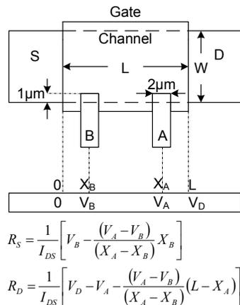
Fig. 6. Gated four-terminal device fabricated to directly measure the contact resistances. Probes A and B use the same type of contact as the S/D, and extend into the channel by  $1\mu\text{m}$ .
