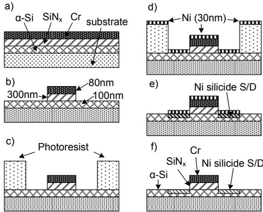
Fig. 1. Illustration of fabrication process: a) Deposition of TFT stack ( $\alpha$ -Si, gate dielectric, and gate metal); b) definition of gate electrode; c) definition of channel width electrical isolation of devices; d) blanket deposition of Ni; e) lift off and silicidation; f) selective removal of unreacted Ni
