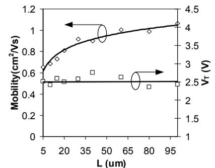
Fig. 8. Simulated and measured channel length dependence of effective mobility and threshold voltage.  $\mu_{\text{eff}}$  is decreased by 30% from its long channel value at  $L = 5\mu\text{m}$ ,  $V_T$  is unchanged.
