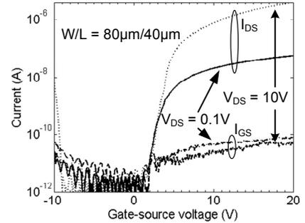
Fig. 2. Room-temperature transfer characteristics (drain current vs gate-source voltage for drain-source bias of 0.1V and 10V) of a top gate a-Si TFT with self-aligned nickel silicide source drain.
