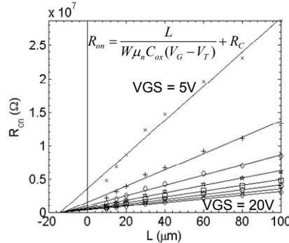
Fig. 4. Total device resistance in the linear regime ( $R_{ON}$ ) as a function of channel length for  $V_{GS}$  ranging from 5V to 20V and fits to model for extracting  $R_C$
