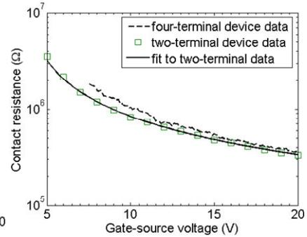
Fig. 5. Contact resistance vs  $V_{GS}$  - two-terminal device data extracted using the approach shown in Fig. 4 and four-terminal device data measured using the approach shown in Fig. 6.
