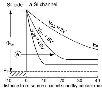
Fig. 7. Band diagram near semiconductor surface from source to channel. Increasing  $V_{GS}$  lowers conduction band and increases electron concentration in the channel, resulting in a thinner tunnel barrier to enable electron injection
