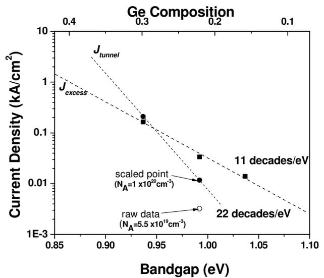
**Fig. 5** Band-to-band tunneling current and excess current (at 0.5V) vs. bandgap energy (Ge composition). For 22% Ge, the experimental point has been scaled to the expected point for boron doping ( $1 \times 10^{20} \text{ cm}^{-3}$ ) using [3]
