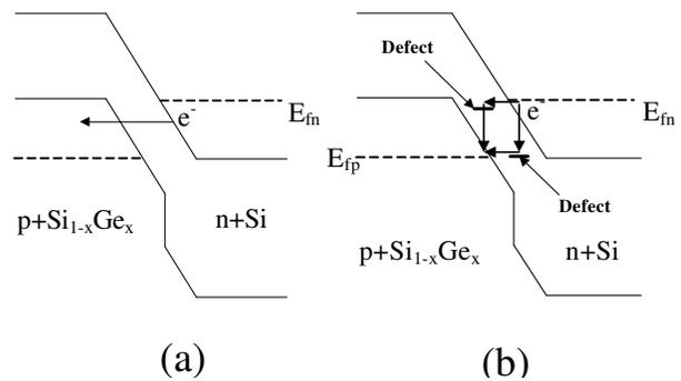
**Fig. 3** Tunneling mechanisms of (a) band-to-band tunneling current and (b) defect-mediated excess current
