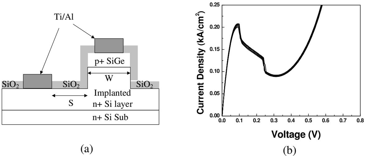
**Fig. 1** (a) Cross section of test  $\text{Si}_{1-x}\text{Ge}_x/\text{Si}$  tunneling diodes; (b) I-V curves of 8  $\text{Si}_{0.7}\text{Ge}_{0.3}/\text{Si}$  tunneling diodes with NDR effect. Side contacts were used to reduce series resistance effect.
