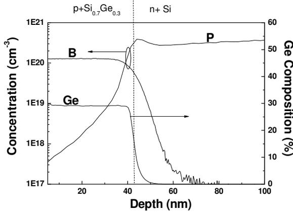
**Fig. 2** Doping profiles and Ge composition vs. depth by SIMS analysis
