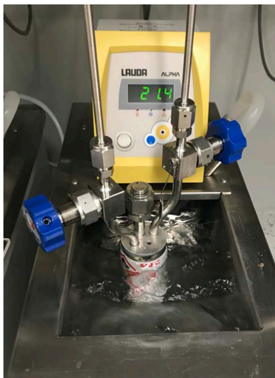
Figure 2.19: Bubbler cylinder for liquid precursor storage, immersed in circulating temperature-controlled water bath.
