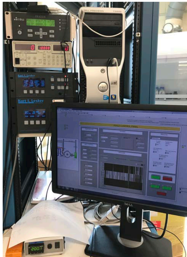
Figure 2.24: PEALD control station showing Labview interface.
