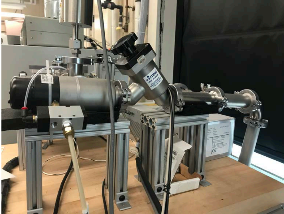
Figure 2.23: Gate valve attached to pilot valve and manual throttle valve. Manometer visible in background; pump beneath table.
