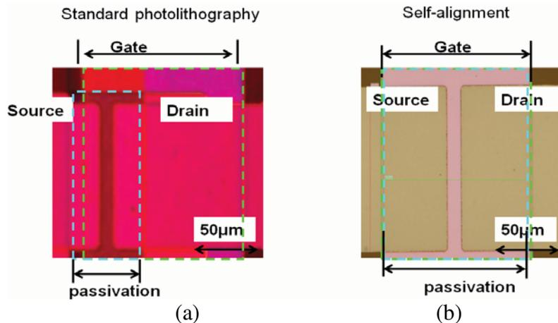
**Figure 4 Optical micrographs showing the alignment between the gate and subsequent layers for (a) a TFT 3cm away from the center of the substrate fabricated using standard patterning, and (b) a TFT which the channel passivation patterned using self-alignment.**
