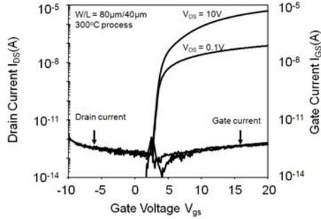
**Figure 3 Transfer characteristics of a self-aligned a-Si:H TFT made on clear plastic at 300°C.**
