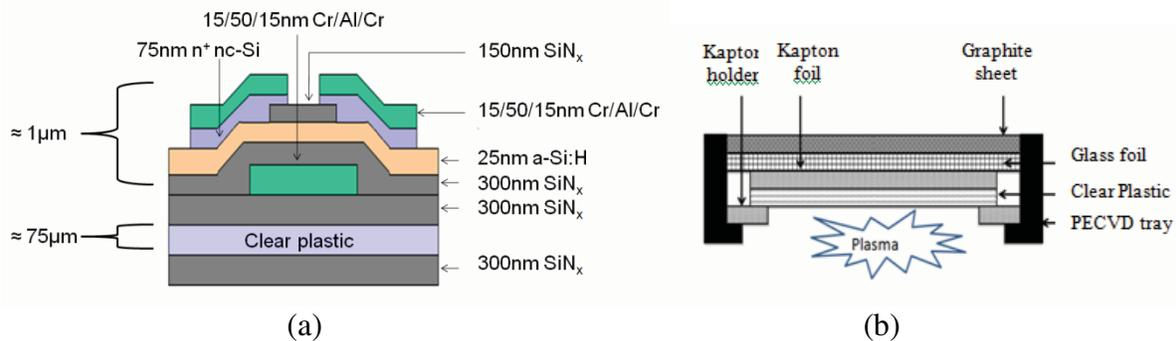
**Figure 1 (a) Schematic of transistor geometry (b) Cross-sectional view of face-down substrate mount for plasma-enhanced chemical vapor deposition.**
