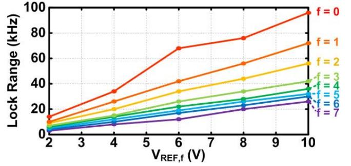
Fig. 17. Simulated lock range versus reference-signal voltage amplitude.
