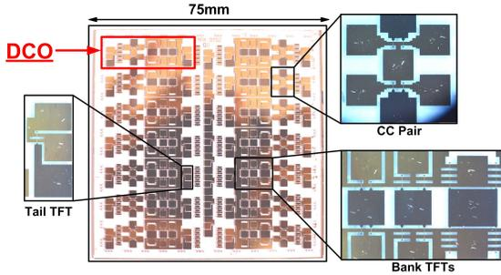
Fig. 23. Photograph of DCO sample, highlighting DCO components.
