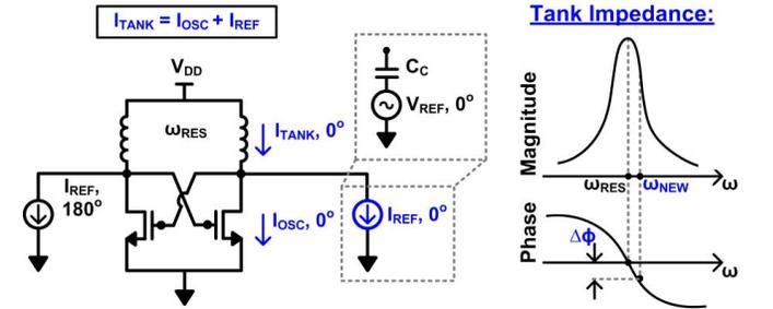
Fig. 14. Injection-locking principle.
