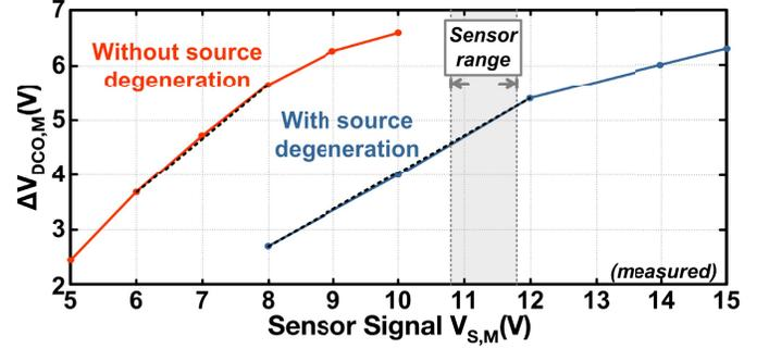
Fig. 13.  $V_{S,M}$ -to- $V_{DCO,M}$  transfer function with and without source degeneration of a tail transistor, showing increased linear range of sensor input. Linear fit within range for each in black.
