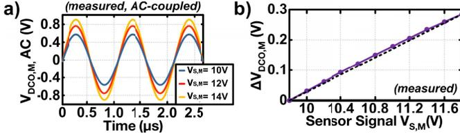
Fig. 12. Measured amplitude modulation of a DCO output  $V_{DCO,M}$  over a range of input sensor signals  $V_{S,M}$ , and (a) time-domain waveform and (b)  $V_{S,M}$ -to- $V_{DCO,M}$  transfer function in purple.
