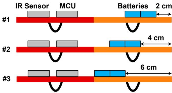
Fig. 11. The three different battery positions we used to study the impact of weight distribution. We define the figures from top to bottom as battery position #1, #2, and #3, respectively. Battery position #1 is the default position used in the majority of tests presented in this paper.
