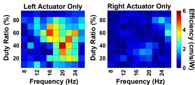
Fig. 14. The actuation efficiency of the robot as a function of frequency and duty ratio when driving only the left actuator (left figure) or the right actuator (right figure). Driving the left actuator is more efficient than driving the right actuator. Carrying the batteries makes the right actuator less efficient. Batteries at position #1.
