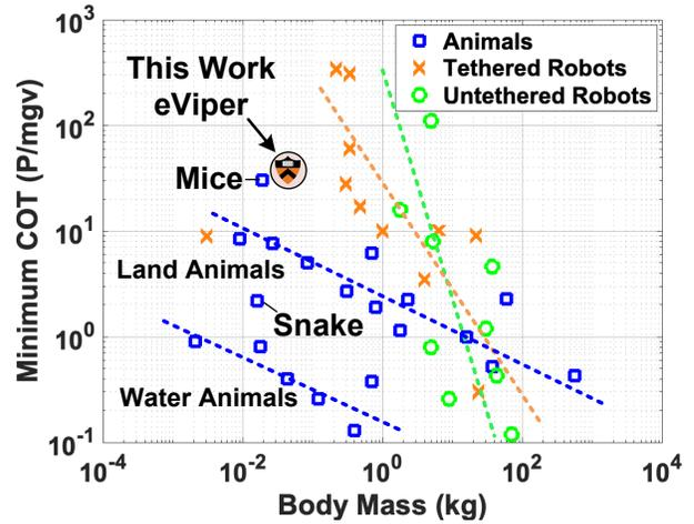
Fig. 21. Cost of transport (COT) of the eViper compared to other published soft or rigid systems. eViper is much lighter than most other untethered robot designs. The lowest COT of the soft eViper is about 36.4 W/(kg·m<sup>2</sup>/s<sup>3</sup>), which is similar to the COT of mice (data from [26]). The dotted lines depict the fitted mass-COT trends for land animals, water animals, tethered robots, and untethered robots.
