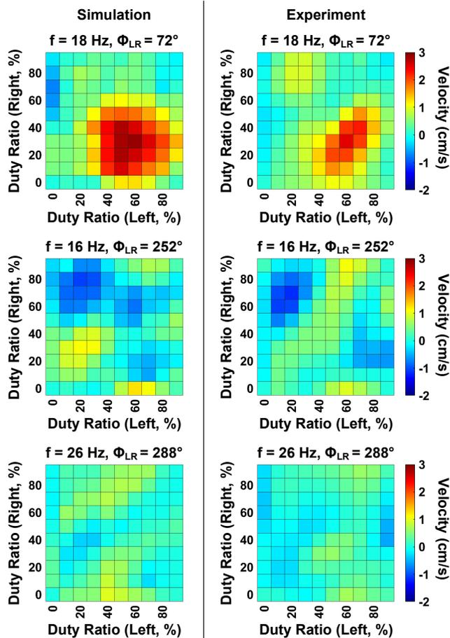
Fig. 17. Simulated (left) and measured (right) soft robot velocity when both actuators are activated. The two actuators are driven at the same frequency  $f$  and a specific phase  $\Phi_{LR}$ , as shown in the title of each graph, but at different duty ratios. Batteries at position #1.
