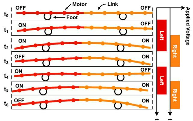
Fig. 9. Illustration showing the concept of the motor-link structure together with several frames ( $t_0$  to  $t_6$ ) in a simulation video. We use five motors to simulate one actuator. The time difference between each frame is 20 ms. The right side shows the applied voltage versus time. The red and orange voltages correspond to the left and right actuator, respectively.
