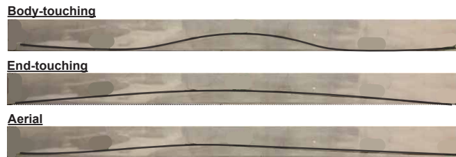
Fig. 14: Three representative experimental shapes for the motion at 14 Hz driving frequency.
