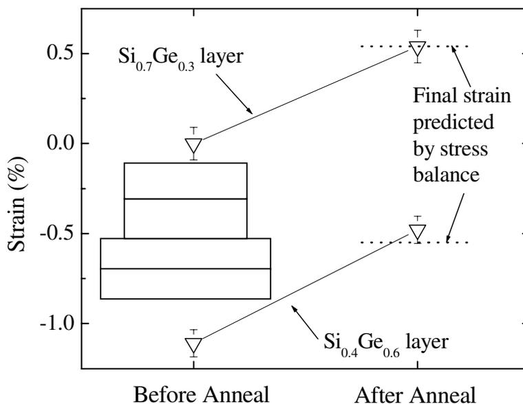
Fig. 3. Biaxial strain of  $\text{Si}_{0.7}\text{Ge}_{0.3}$  and  $\text{Si}_{0.4}\text{Ge}_{0.6}$ , measured by Raman spectroscopy at the center of a  $20\ \mu\text{m} \times 20\ \mu\text{m}$  island, before and after 20-min annealing at  $800^\circ\text{C}$ . Open symbols are experimental data and dotted lines are based on calculation of stress balance.
