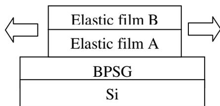
Fig. 1. Schematic of stress balance between elastic films on BPSG. During high-temperature annealing, the BPSG softens and the effectively freestanding elastic films minimize strain energy by lateral displacement. The equilibrium state is governed by net zero stress.
