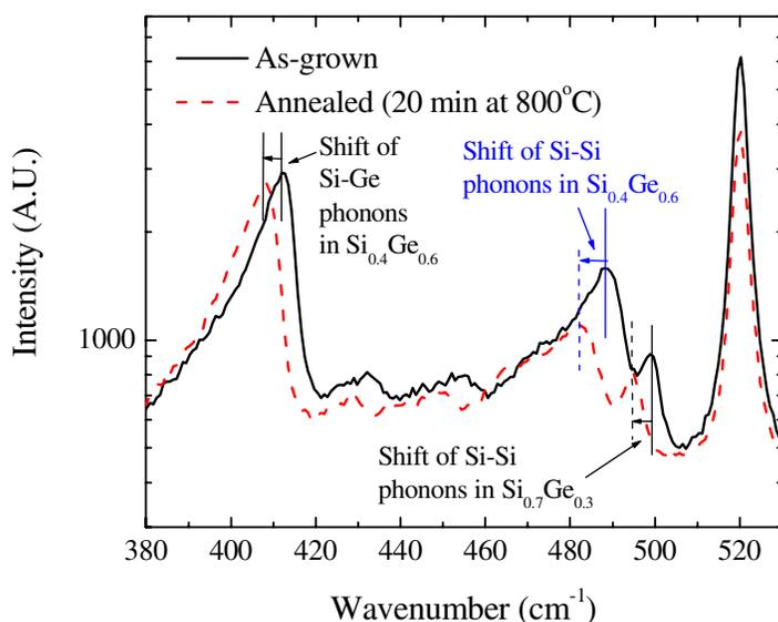
Fig. 2. Raman spectrum, measured at the center of a 20  $\mu\text{m}$  x 20  $\mu\text{m}$  island comprising 30nm  $\text{Si}_{0.4}\text{Ge}_{0.6}$ /30nm  $\text{Si}_{0.7}\text{Ge}_{0.3}$ , before and after 800°C annealing for 20 min. All phonon peaks from both films shift toward lower wavenumbers after an annealing to reach stress balance, consistent with coherent lateral expansion of the island.
