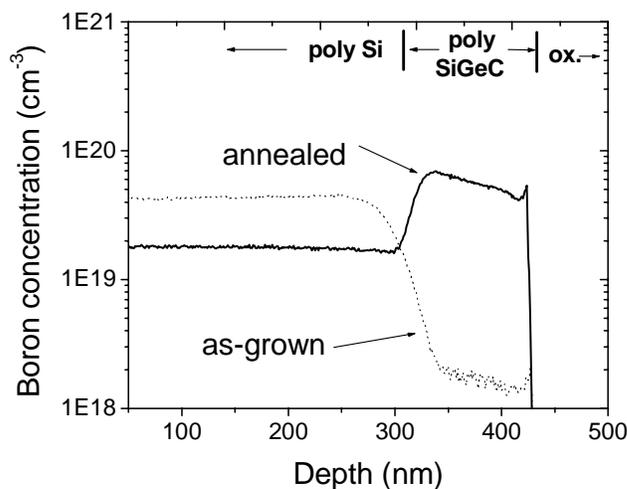
Figure 1: SIMS profiles of boron concentration in two-layer structure before and after annealing at 800°C for 44 hours in N<sub>2</sub>.
