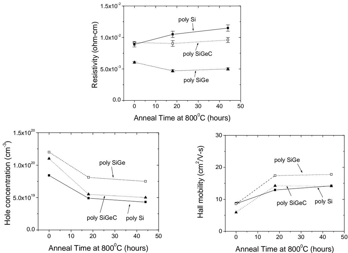
Figure 3: Resistivity, hall mobility, and hall concentration vs. anneal time at  $800^\circ\text{C}$  for single in-situ doped layers ( $[\text{B}] \sim 10^{20}$  atoms/ $\text{cm}^3$ ) of poly Si, SiGe, and SiGeC.
