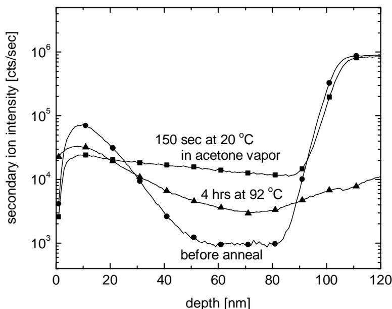
**Figure 4.** SIMS profile of a sample with C6 transferred into a PVK film before (squares) and after (circles) acetone anneal. The sample was annealed in acetone vapor for 150 sec at room temperature. For comparison, a thermally annealed sample (4 hours at 92 °C) after the same initial transfer is also shown (triangles).
