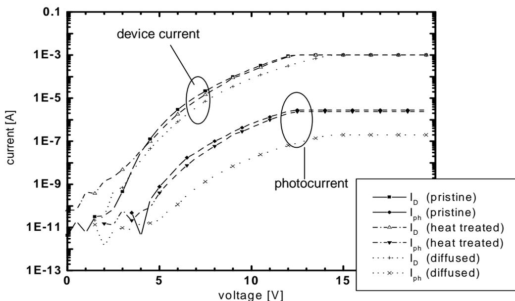
**Figure 2.** IV-characteristics and photocurrents of different devices: (a) a device (PVK/PBD/C6) which was not exposed to heat at all, (b) a device (PVK/PBD/C6) which was kept at 70 °C for 1 hour in vacuum, and (c) a device (PVK/PBD only) with diffused C6 at 70 °C for 1 hour in vacuum [10].
