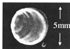
Fig. 7. Acetone:C6 Deposition. (a) Droplet radius with time during evaporation. (b) Photoluminescence of dye doping, where brightness corresponds to C6 concentration.
