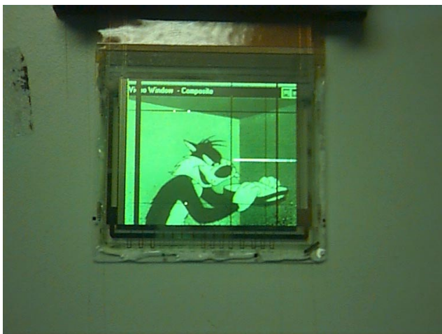
Fig. 9. QVGA Display showing video operation.
