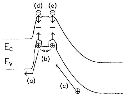
FIG. 9. Schematic band diagram showing the source of the two base currents  $I_{B1}$  and  $I_{B2}$ .
