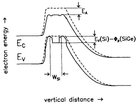
FIG. 10. Band diagram of DBHBT (solid lines) and Si homojunction transistor (dashed lines) showing the parameters determined from electrical measurements: barrier thickness  $W_{Si}$ ; effective band gap reduction  $E_A$ ; and barrier height for holes,  $E_V(Si) - \Phi_p(SiGe)$ .
