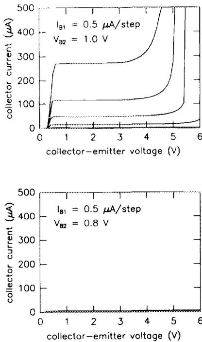
FIG. 7. Common-emitter characteristics (with input current into base 1) of DBHBT at 85 K for  $V_{B2}$  of (a) 1.0 V, and (b) 0.8 V showing control of the current gain  $I_C/I_{B1}$  by the voltage applied at the second base.
