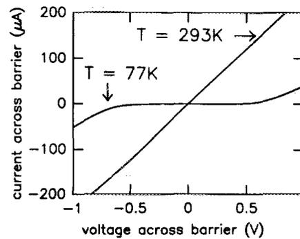
FIG. 5. Current-voltage characteristics of the  $p$ -Si<sub>1-x</sub>Ge<sub>x</sub>/ $i$ -Si/ $p$ -Si<sub>1-x</sub>Ge<sub>x</sub> barrier of device No. 1077 at room temperature and at 77 K.
