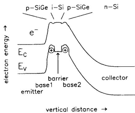
FIG. 1. Calculated band diagram of DBHBT, obtained by inserting an intrinsic silicon layer into the  $p$ -Si<sub>1-x</sub>Ge<sub>x</sub> base of a flat-base HBT. Note that the conduction band in the base is still approximately flat because  $\Delta E_c \ll \Delta E_v$  at the Si/Si<sub>1-x</sub>Ge<sub>x</sub> heterojunction.
