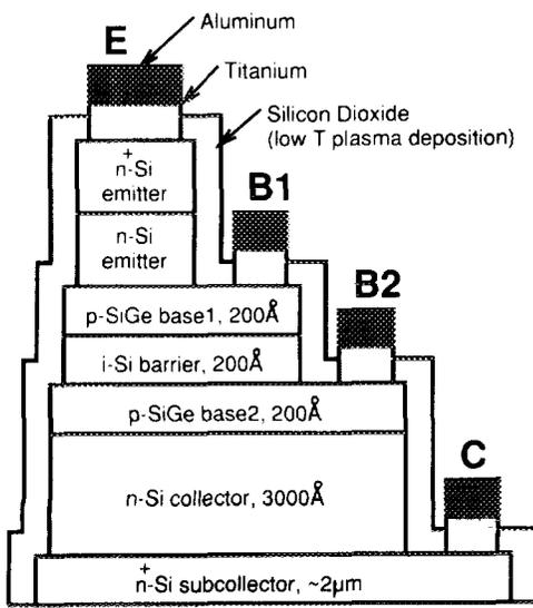
FIG. 3. Triple mesa device structure of DBHBT.
