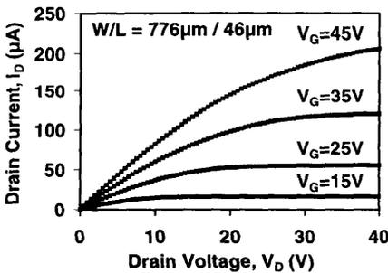
Figure 3. Transfer characteristics of TFT on 75 μm steel foil.
