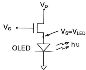
Figure 6b. Equivalent circuit for TFT/OLED.
