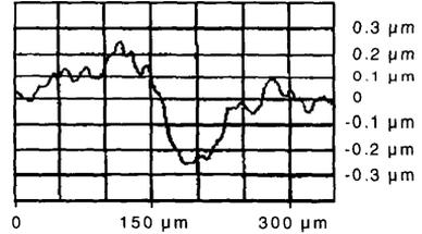
Figure 1b. Surface profile of "planarized" 75  $\mu\text{m}$  foil.
