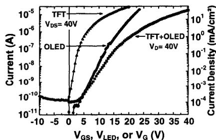
Figure 7. *I-V characteristics of the TFT, the OLED and the integrated TFT/OLED.*
