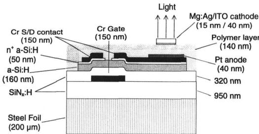
Figure 6a. Schematic cross section of integrated TFT/OLED.
