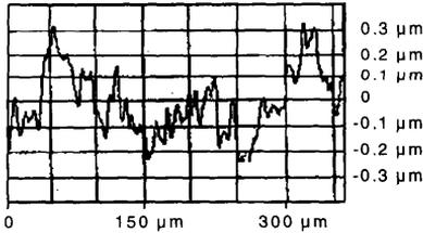
Figure 1a. Surface profile of as-rolled 75  $\mu\text{m}$  foil.
