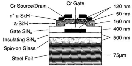
Figure 2. Schematic cross-section of TFT on 75 μm steel foil.
