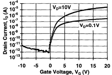
Figure 4. Output characteristics of TFT on 75 μm steel foil.
