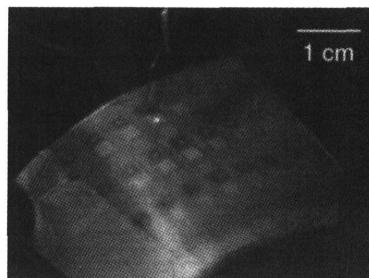
Figure 9. *The operation of the integrated TFT/OLED (bright spot) on the steel foil in the bent configuration.*
