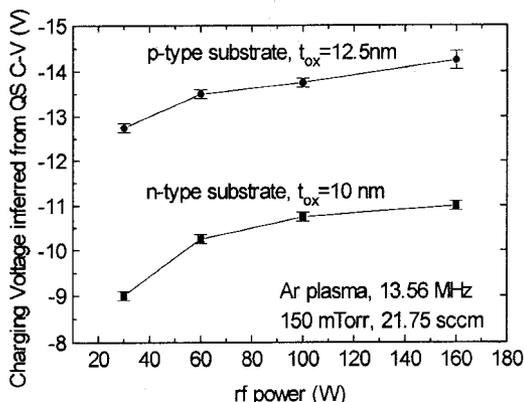
Fig. 7. Charging voltage inferred from DC bias stressing and matching the QS C-V curves for n & p type substrate MOS capacitors.
