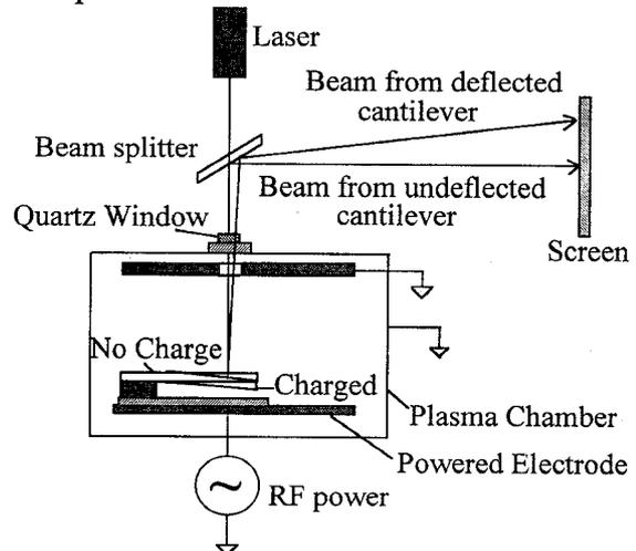
Fig. 3. Experimental setup used to detect charge in plasma, showing reflected beam from charged and uncharged sensor.
