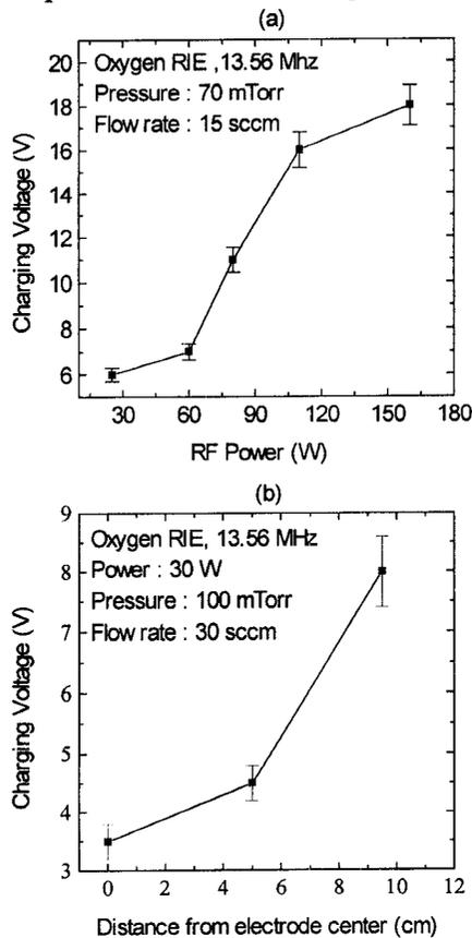
Fig. 4. (a) Charging Voltage as a function of input rf power, (b) Charging Voltage as a function of position on the electrode.
