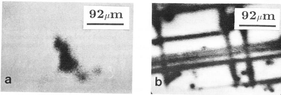
Figure 2. Monochromatic CL images recorded at  $T \approx 5$  K,  $E_o = 10$  keV,  $I_b = 0.1$  nA, a) QW  $\text{Si}_{0.8}\text{Ge}_{0.2}$ , thickness 33 Å, b) QW  $\text{Si}_{0.8}\text{Ge}_{0.2}$ , thickness 500 Å.
