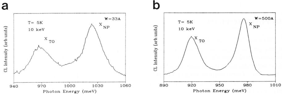
Figure 1. CL spectra recorded at  $T\approx 5\text{ K}$ ,  $E_o=10\text{ keV}$ ,  $I_b=0.1\text{ nA}$ , a) QW  $\text{Si}_{0.8}\text{Ge}_{0.2}$ , thickness  $33\text{ \AA}$ , b) QW  $\text{Si}_{0.8}\text{Ge}_{0.2}$ , thickness  $500\text{ \AA}$ .
