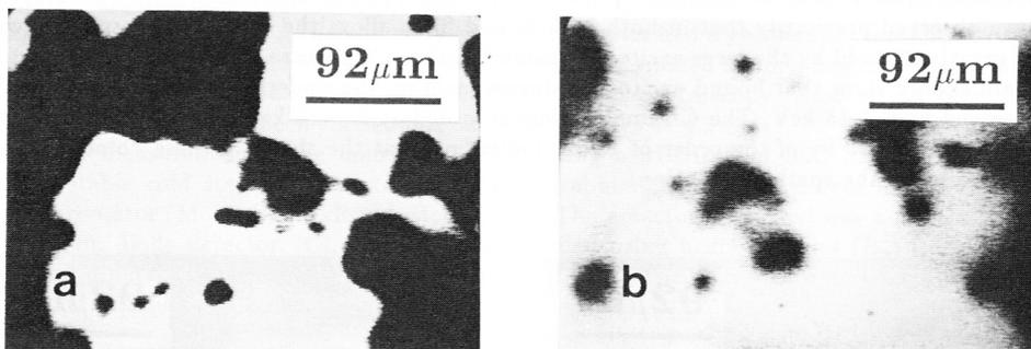
Figure 3. Monochromatic CL images recorded of the SiGe 500 Å sample, a) Annealing for 1 hour at  $T=300^{\circ}\text{C}$ , b) same treatment as a) different area.
