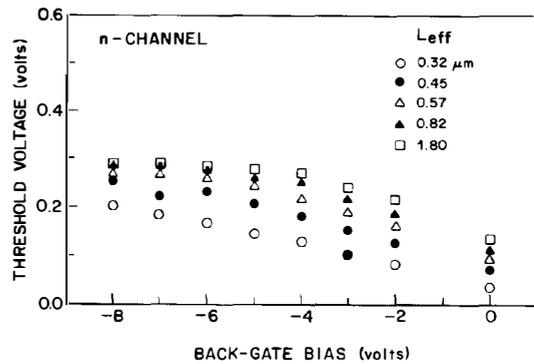
Fig. 4 Threshold voltage of n-channel devices as a function of back-gate bias.
