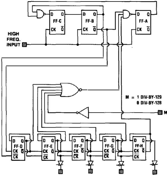
Fig. 2 CMOS prescaler functional block diagram.
