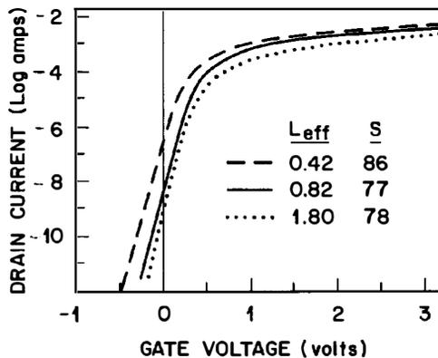
Fig. 6 Subthreshold behavior of 3 transistors with design gate lengths of  $0.62 \mu\text{m}$ ,  $1.0 \mu\text{m}$  and  $2.0 \mu\text{m}$ .  $V_{ds} = 0.01 \text{ V}$ . The  $L_{eff}$  is given in  $\mu\text{m}$ , and  $S$ , the subthreshold swing, in  $\text{mV}/\text{decade}$ .
