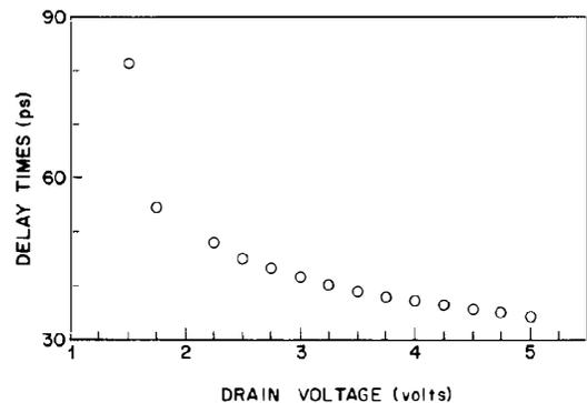
Fig. 8 Ring oscillator delay times as a function of drain voltage.
