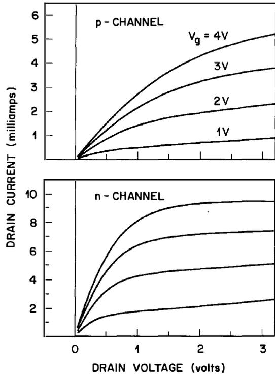
Fig. 3 Drain current vs. voltage characteristics of 0.62  $\mu$ m ( $L_{eff}=0.42\mu$ m) n- and p-channel transistors with -6V back-gate bias.
