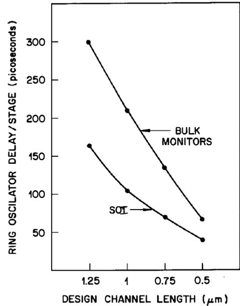
Fig. 7 The ring oscillator delays as a function of gate length for both SOI and the bulk monitors.
