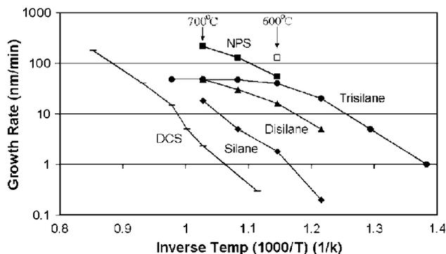
**Figure 2.** Comparison of low-pressure chemical vapour deposition (LPCVD) epitaxial growth rates versus inverse temperature for sources of dichlorosilane (DCS), silane, disilane, trisilane [6, 7] and novel neopentasilane (NPS) precursor on (100) silicon substrates.
