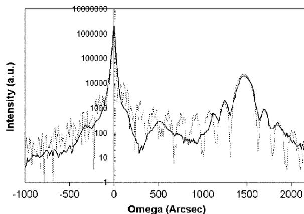
**Figure 3.** High-resolution x-ray diffraction (HR-XRD) of a 130 nm  $\text{Si}_{1-y}\text{C}_y$  layer on Si showing a substitutional carbon level of 1.8% with a lattice constant of 5.375 Å. The solid line represents the raw data while the dotted lines indicate simulation. The growth temperature was 575 °C and the growth rate was 20 nm min<sup>-1</sup>.
