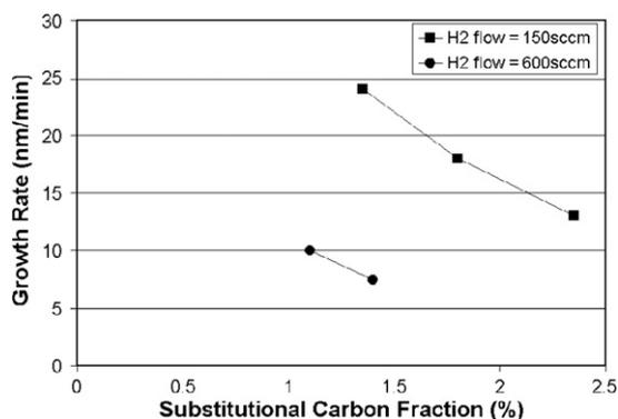
**Figure 6.** Plot of substitutional carbon % versus growth rate. Growth conditions were at 6 Torr. and 575 °C, with constant methylsilane flow of 1 sccm. The squares represent a hydrogen flow of 150 sccm, and the circles represent a hydrogen flow of 600 sccm. The decrease in growth rate is due to a decrease in the NPS source flow.
