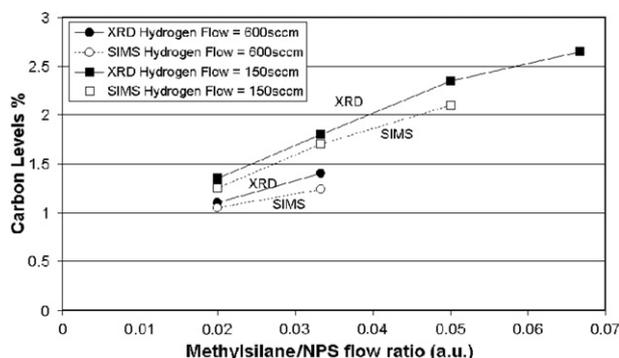
**Figure 4.** Carbon percentage determined by SIMS and calculated from XRD data versus the ratio of methylsilane to NPS source flow at fixed hydrogen flow. The squares represent hydrogen flow of 150 sccm and circles represent hydrogen flow of 600 sccm.
